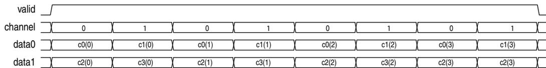
Notice that the channel signal remains a single wire, not a wire for each data wire. It counts from 0 to *ChanCycleCount*-1. Figure 4-13 shows the case with four channels simultaneously on four wires.
