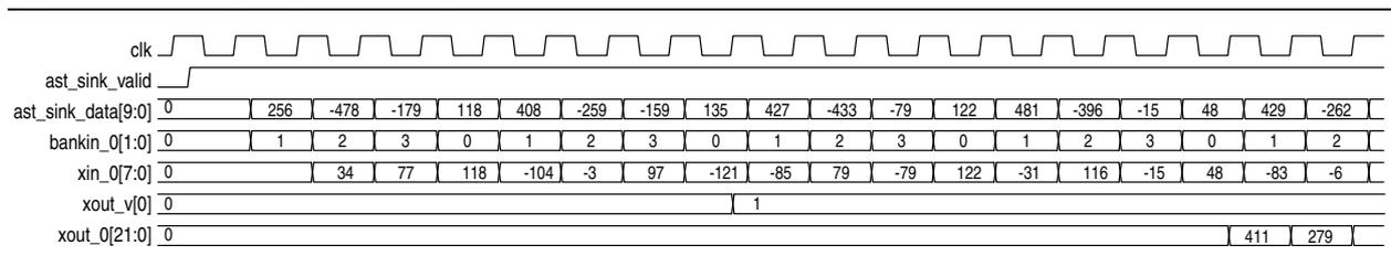
Figure 4-29 shows a timing diagram for a four-channel filter with four coefficient banks and each channel has a separate corresponding coefficient set. The bank inputs for different channels are driven with their channel number respectively throughout the filter operation.
