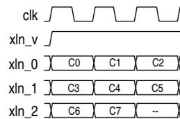
Figure 4-15 shows the expected output format for eight channels on three wires.
