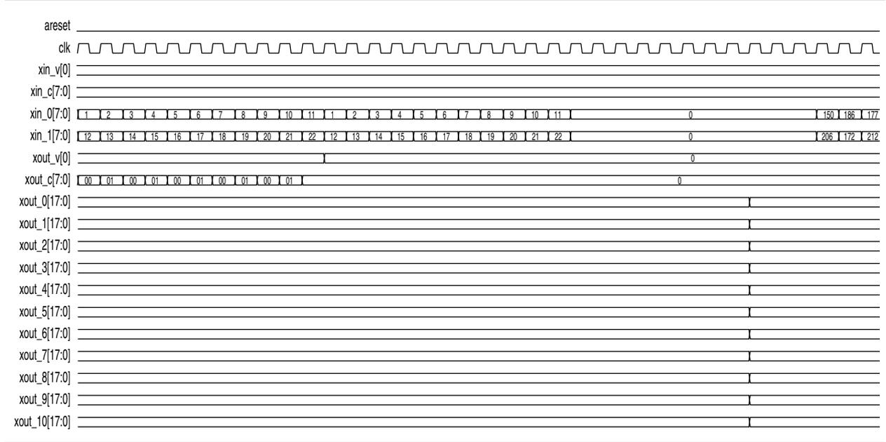
**Figure 4-25. Correct Input Format (11 valid cycles, 11 invalid cycles)**
