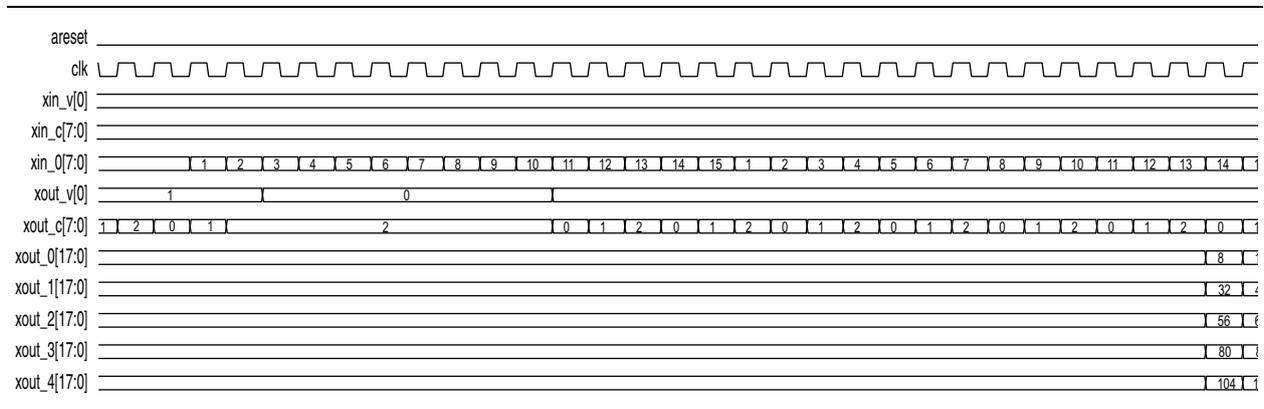
**Figure 4-24. Incorrect Input Format (11 valid cycles, 0 invalid cycles)**
