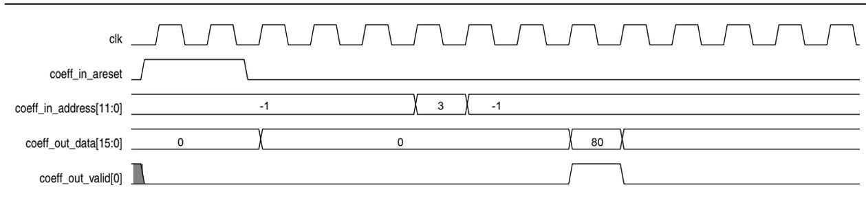
Figure 4-33 shows the timing diagram of a filter with multiple coefficient banks and writable coefficients. It is a symmetry, 13-tap filter. The coefficients data of bank 1 (address 7-13) is reloaded while the filter is running on bank 0. When the coefficient reloading is completed, bank 1 is used to produce an impulse response of the filter and the new coefficient data (-58,18,106...) from bank 1 can be observed on the filter output.
