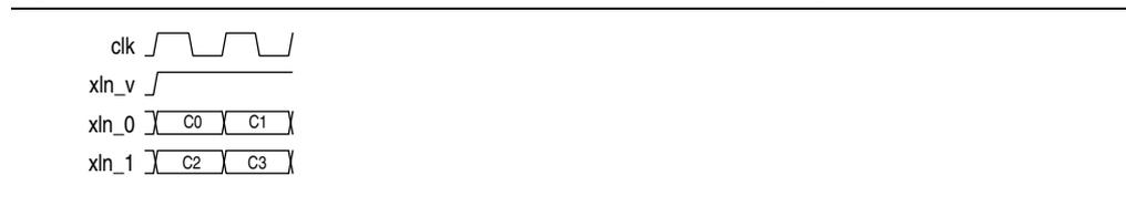
**Figure 4-19. Four Channels on Four Wires with Double Clock Rate (Output)**
