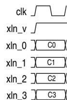
Figure 4-17 shows the expected output format for four channels on four wires.
