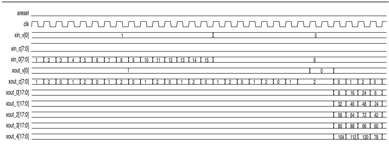
**Figure 4-21. Incorrect Input Format (15 valid cycles, 0 invalid cycles)**
