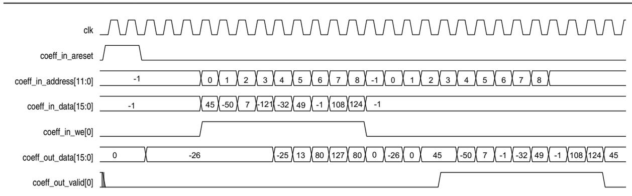
Figure 4-31 shows the timing diagram of a coefficient reloading configuration in Write mode. In this mode, one coefficient data is reloaded. The new coefficient data (123) is loaded into a single address (7).
