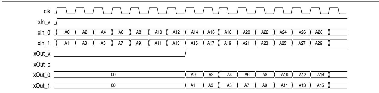
If *inputChannelNum* = 2, then the expected input format is shown in Figure 4-27.
