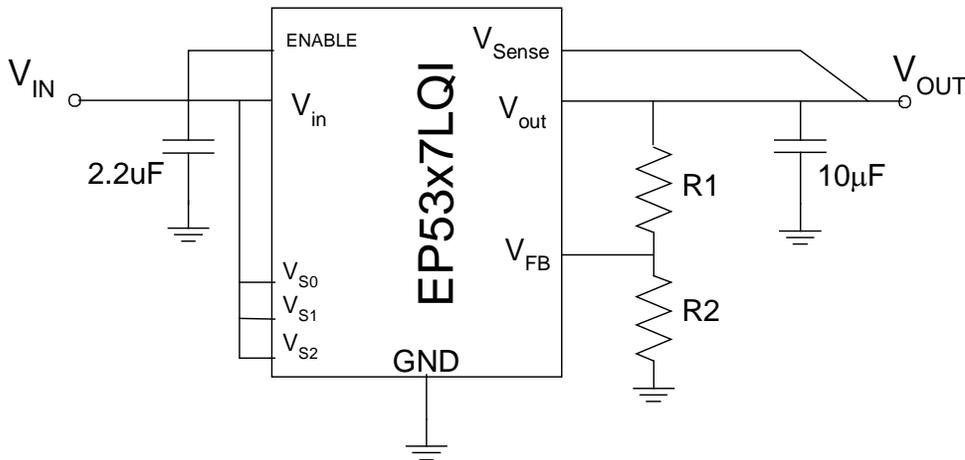
**Figure 3. External divider schematic for the EP53x7LQI**
