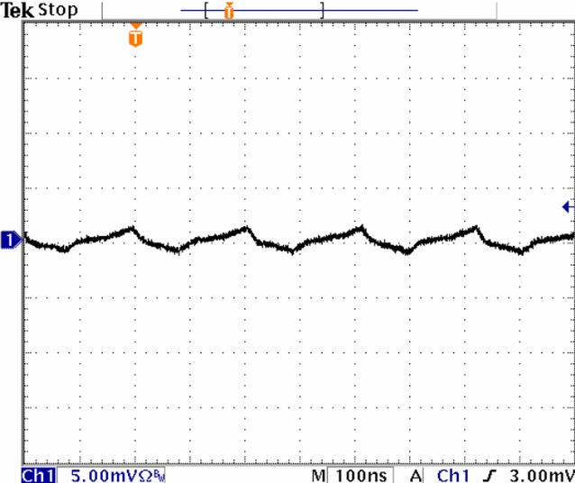
Output Ripple:  $V_{IN} = 3.3V$ ,  $V_{OUT} = 1.8V$
