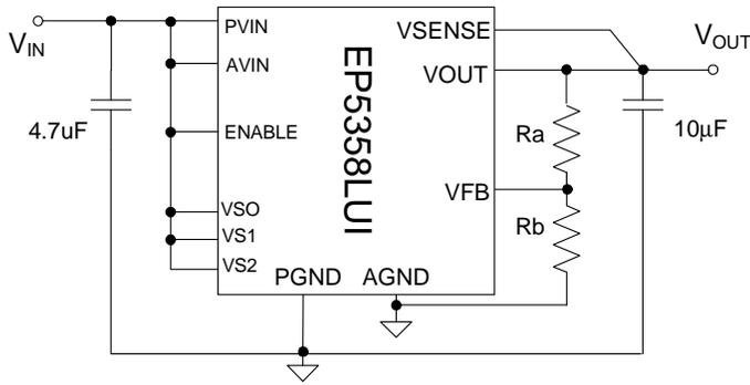
Figure 8: EP5358LUI using external divider
