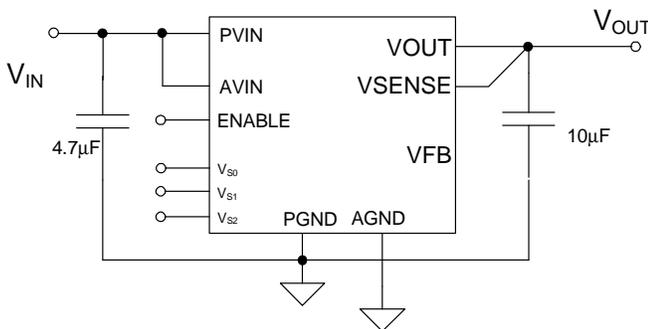
Figure 7: Application Circuit, EP5358LUI, showing the  $V_{FB}$  function.
