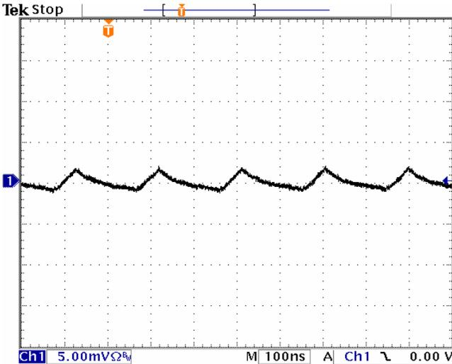
Output Ripple:  $V_{IN} = 5.0V$ ,  $V_{OUT} = 1.2V$ ,
