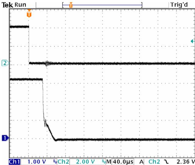
Shut-down Waveform:  $V_{IN} = 5.0V$ ,  $V_{OUT} = 3.3V$ ;
