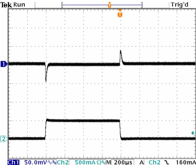
Load Transient:  $V_{IN} = 5.0V$ ,  $V_{OUT} = 1.2V$
