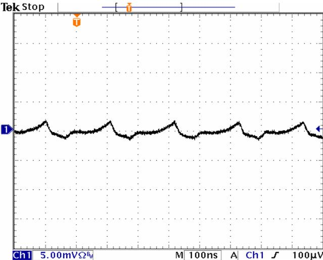
Output Ripple:  $V_{IN} = 5.0V$ ,  $V_{OUT} = 3.3V$
