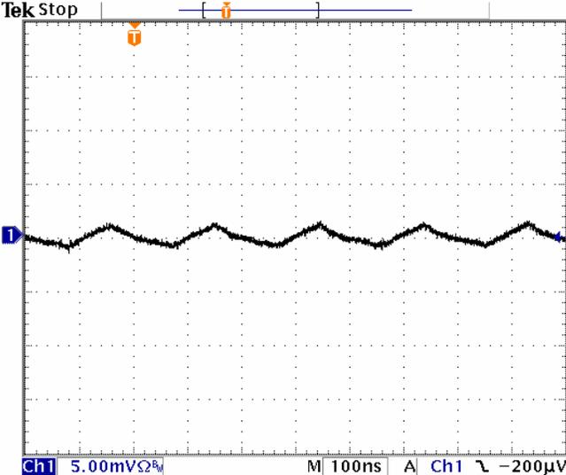
Output Ripple:  $V_{IN} = 3.3V$ ,  $V_{OUT} = 1.2V$ ,
