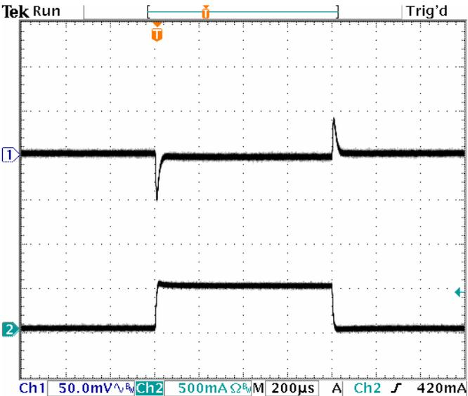
Load Transient:  $V_{IN} = 3.3V$ ,  $V_{OUT} = 1.8V$
