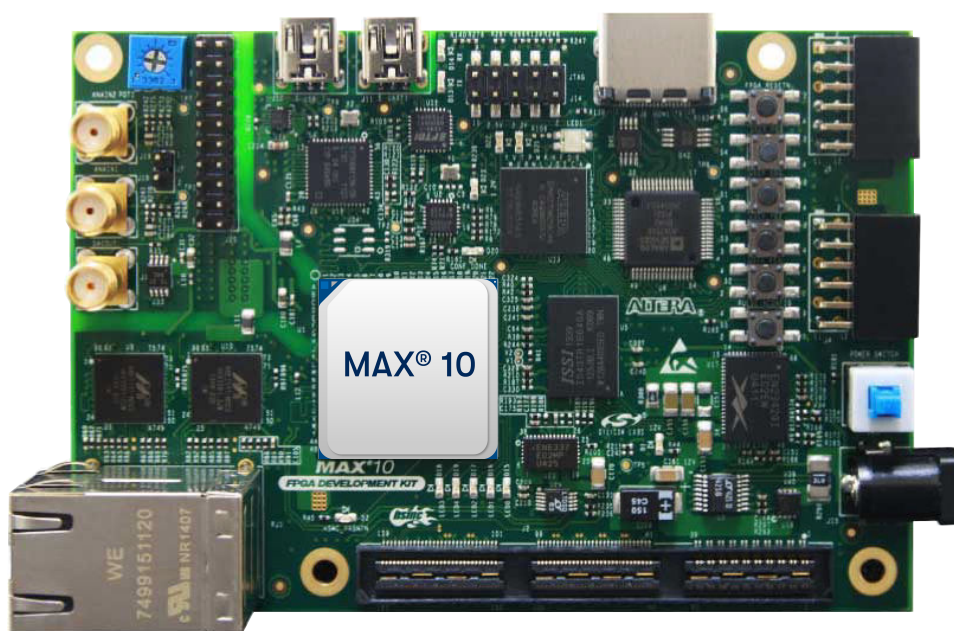
Figure 1. MAX 10 FPGA Development Kit—Top View
