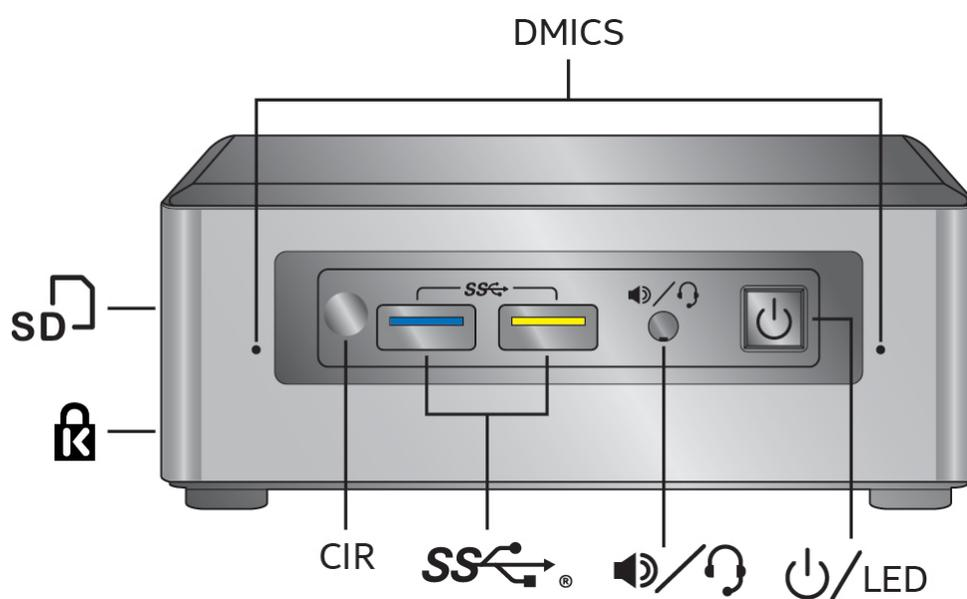
Figure 22. Intel NUC Kit NUC7i5BNH/NUC7i7BNH Features – Front
