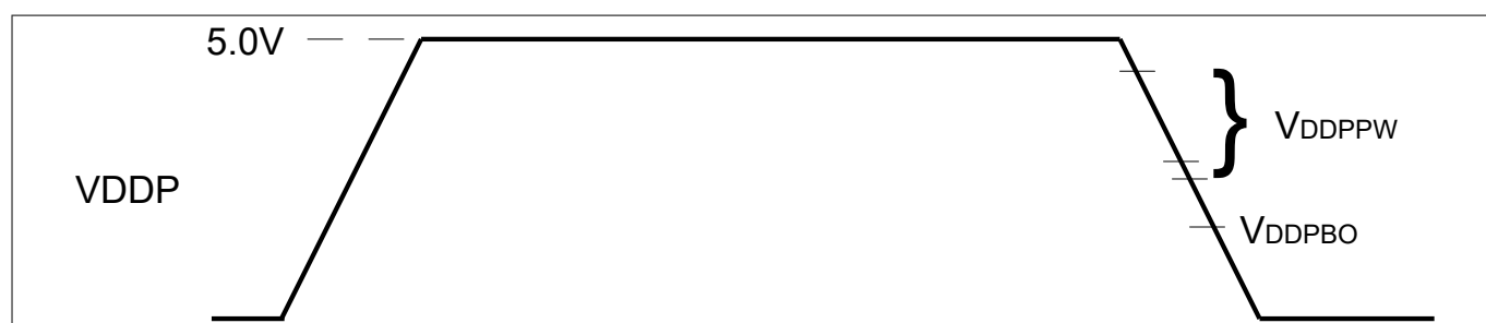
Figure 25 Supply Threshold Parameters
