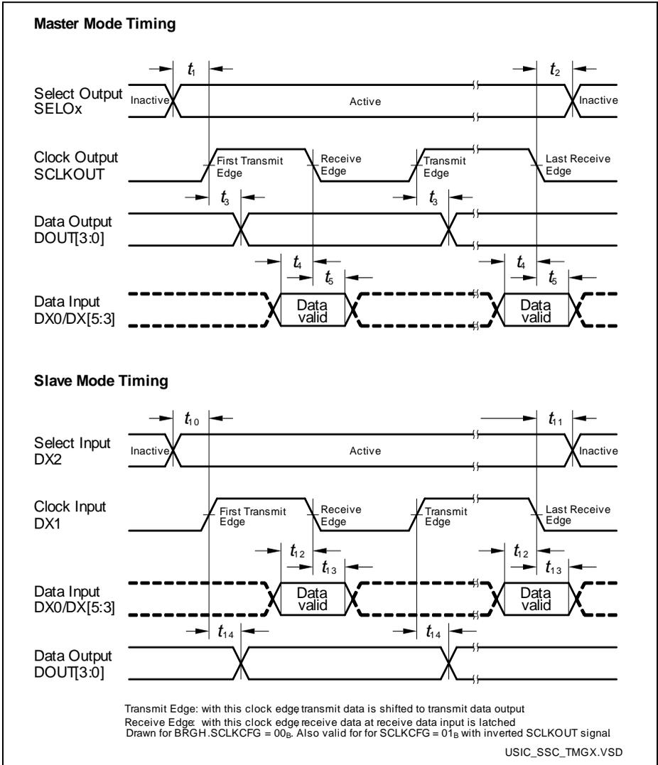
**Figure 22 USIC - SSC Master/Slave Mode Timing**
