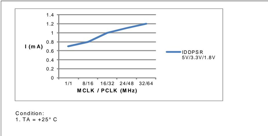
**Figure 15 Sleep mode, peripherals clocks disabled, Flash powered down:
