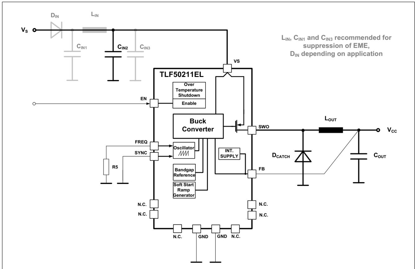
Figure 8 Application diagram
