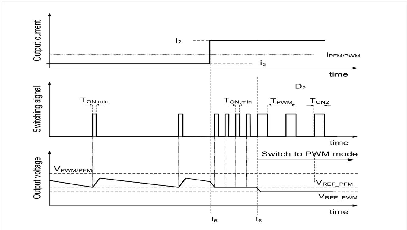
Figure 5 PFM to PWM transition (timing diagram)
