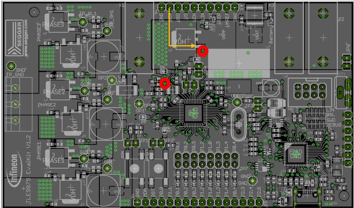
*Note: The disconnected Transistor T1 can cause a voltage drop from VBAT connection to VDHT voltage level. This voltage drop can be avoided by manually connecting the Gate Pin of T1 to the VCP voltage Pin (orange arrow).*
