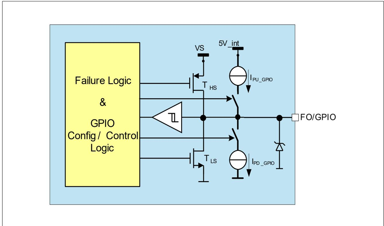
Figure 35 Simplified Fail Output and GPIO Block Diagram
