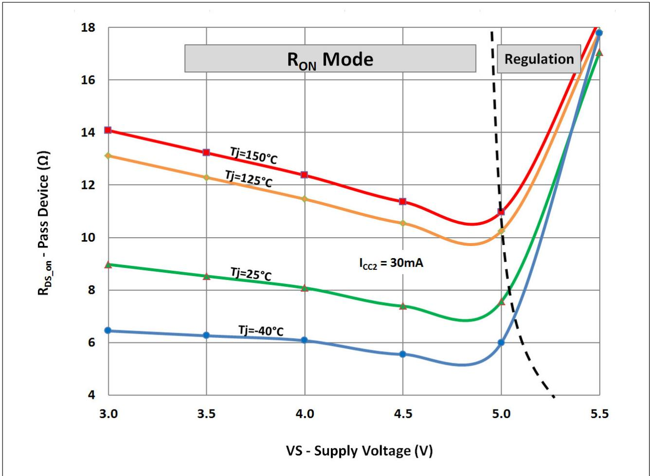
Figure 21 Typical on-resistance of VCC2 pass device during linear (R<sub>ON</sub>) mode for I<sub>CC2</sub> = 30mA
