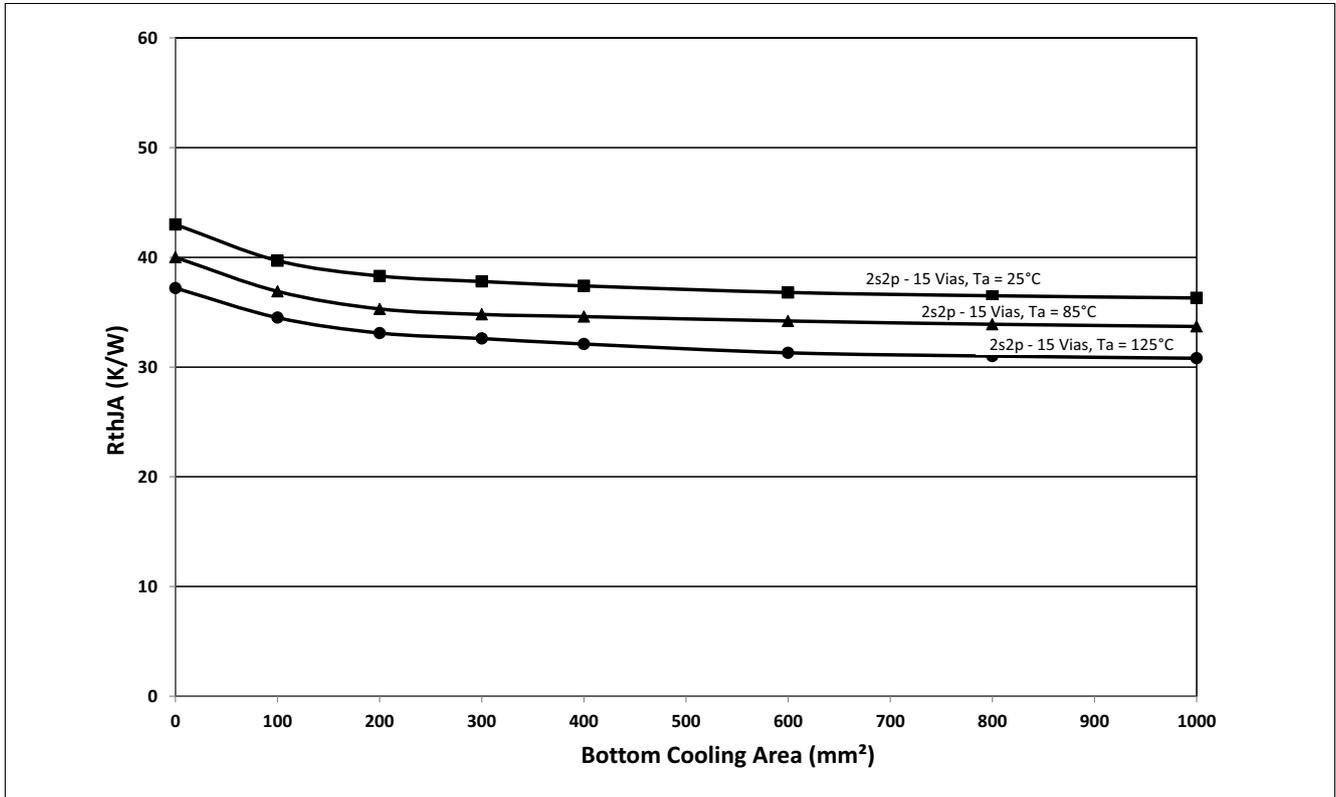
Figure 54 Thermal Resistance ( $R_{th\_JA}$ ) vs. Cooling Area
