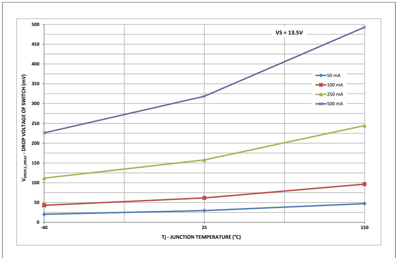
Figure 13 Typical Drop Voltage Characteristics of switch S\_MEAS (between WK/VSENSE & FO/GPIO)
