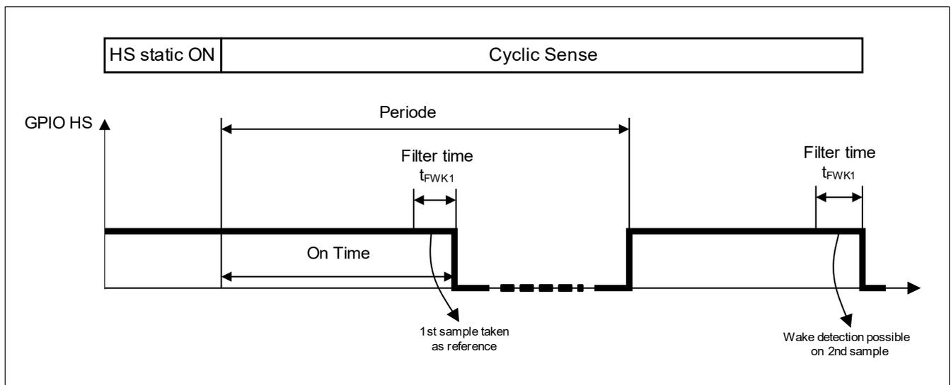
**Figure 8 Cyclic Sense Timing**
