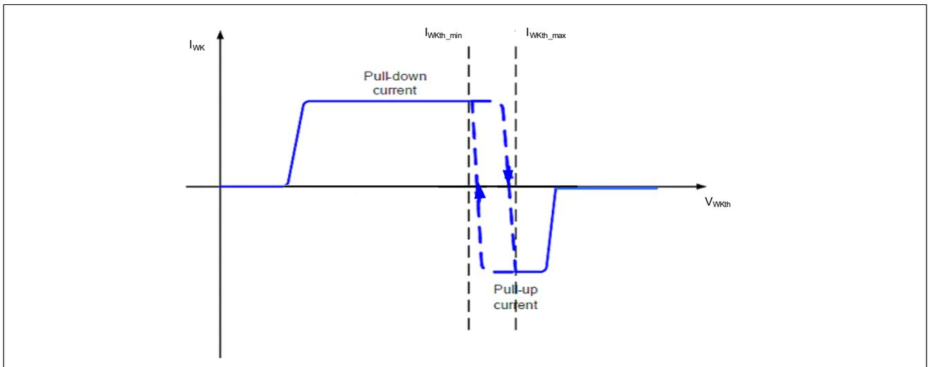
Figure 32 Illustration for Pull-Up / Down Current Sources with Automatic Switching Configuration
