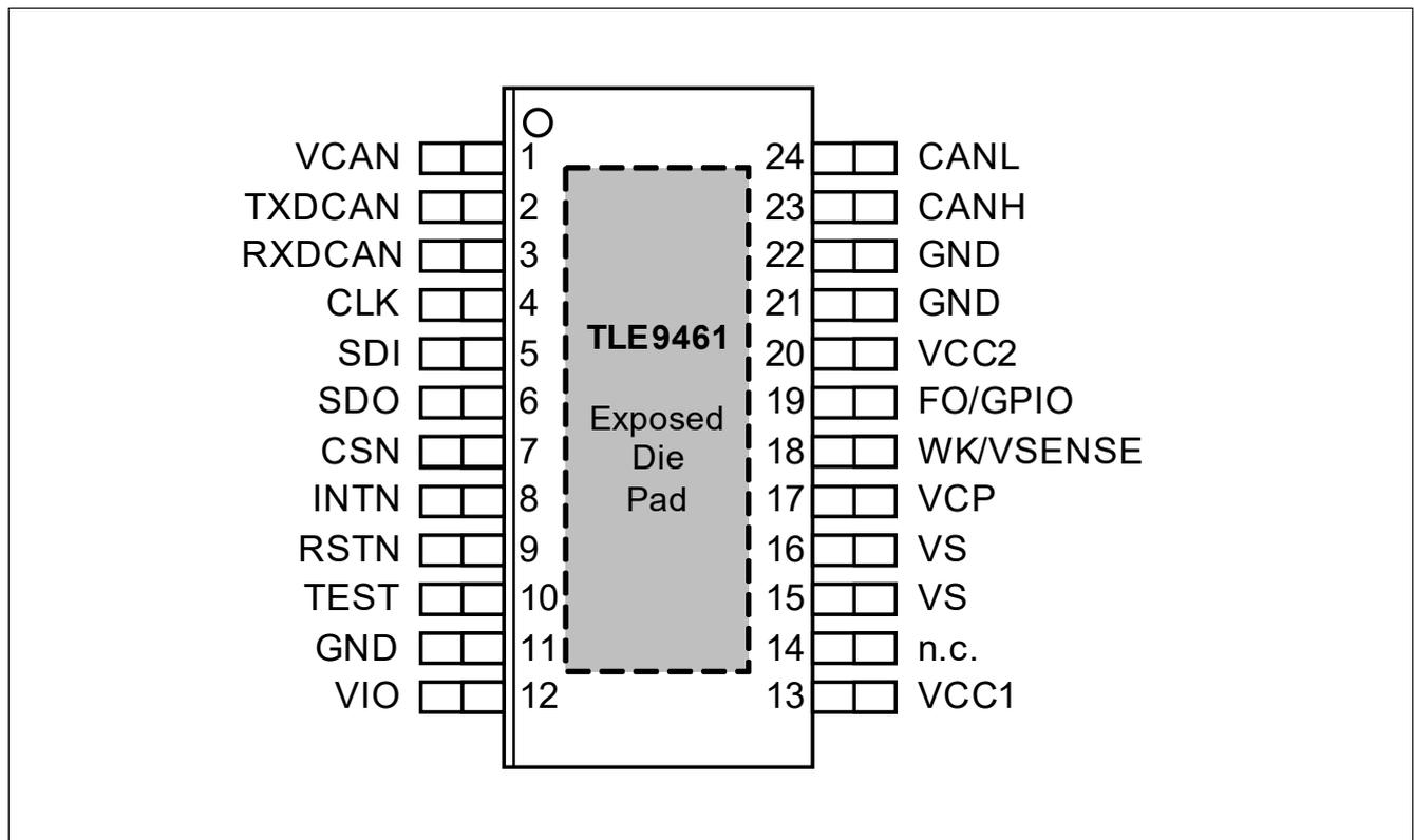
Figure 2 Pin Configuration
