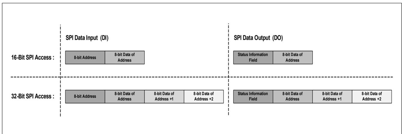
Figure 46 Data access for 16- and 32-bit SPI commands
