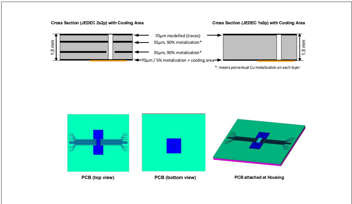
Figure 55 Board Setup
