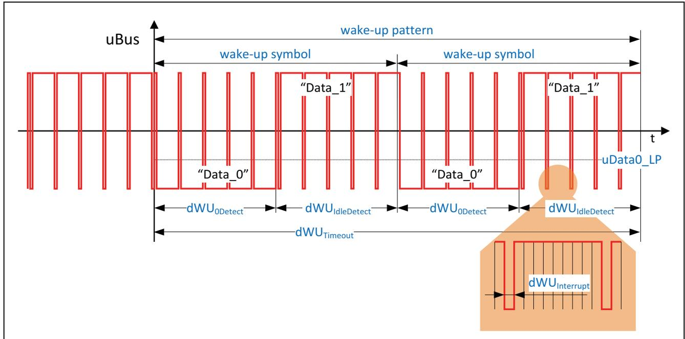
**Figure 20** Wake-up by payload
