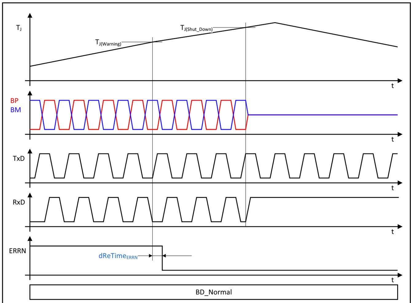
Figure 38 Overtemperature protection
