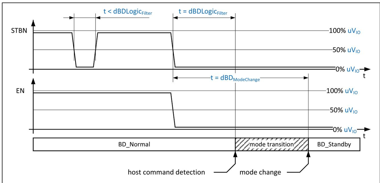
**Figure 10 Example of a valid host command**
