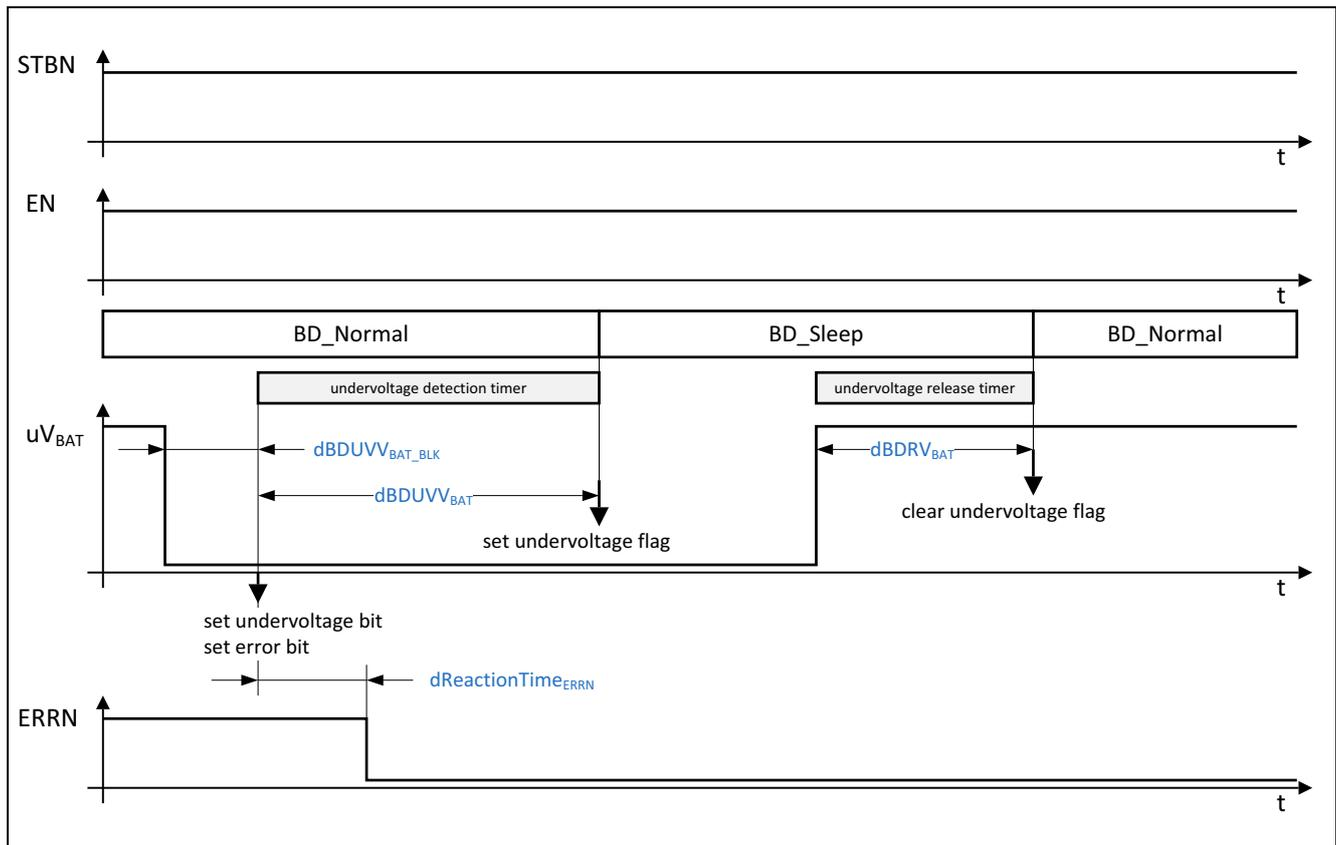
Figure 25 Example of setting the undervoltage flag
