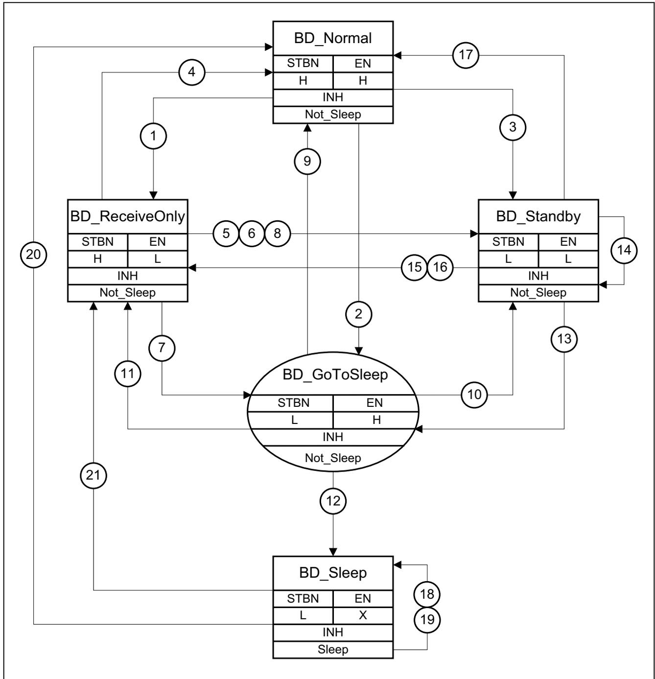
Figure 32 Operating mode change by host command
