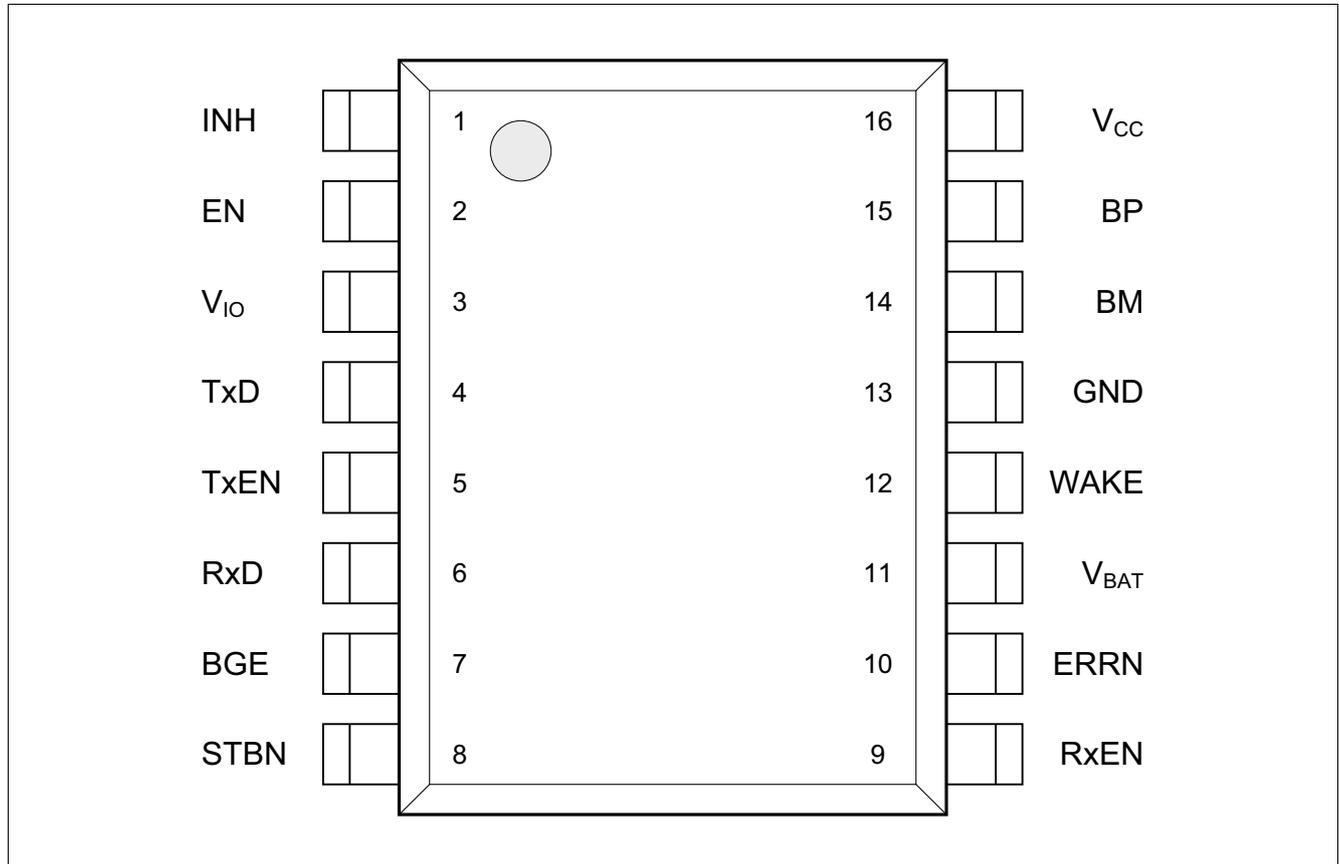
Figure 2 Pin configuration
