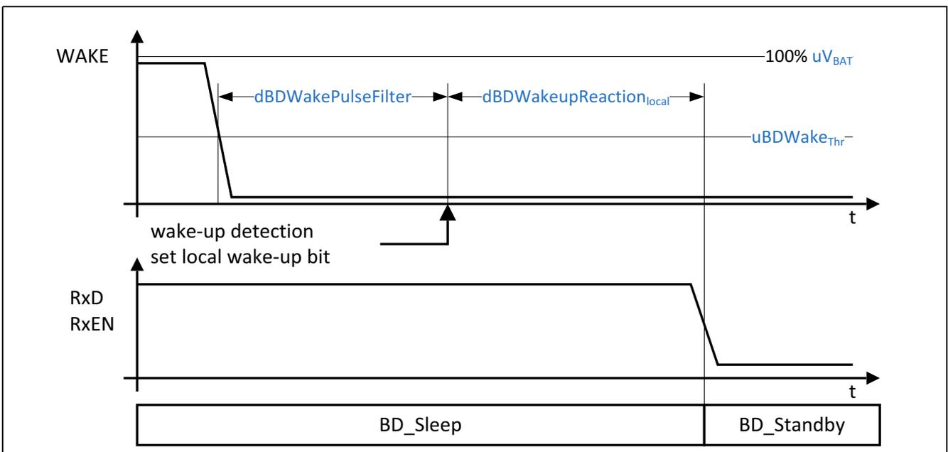
Figure 16 Local wake-up falling edge
