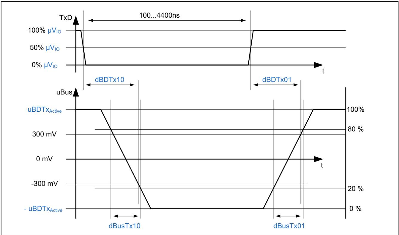
Figure 41 Transmitter characteristics
