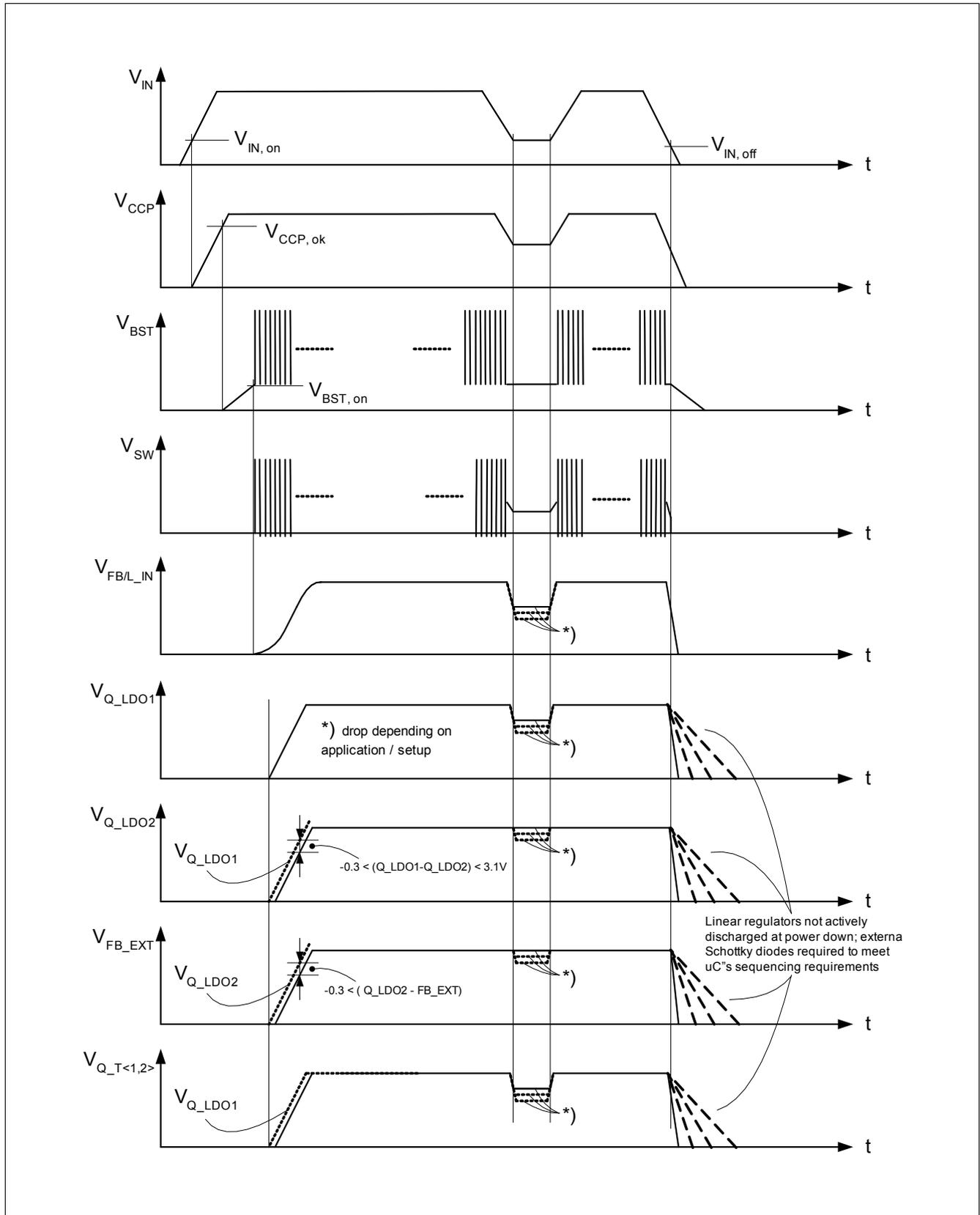
**Figure 4 Power Sequencing of the TLE7368**
