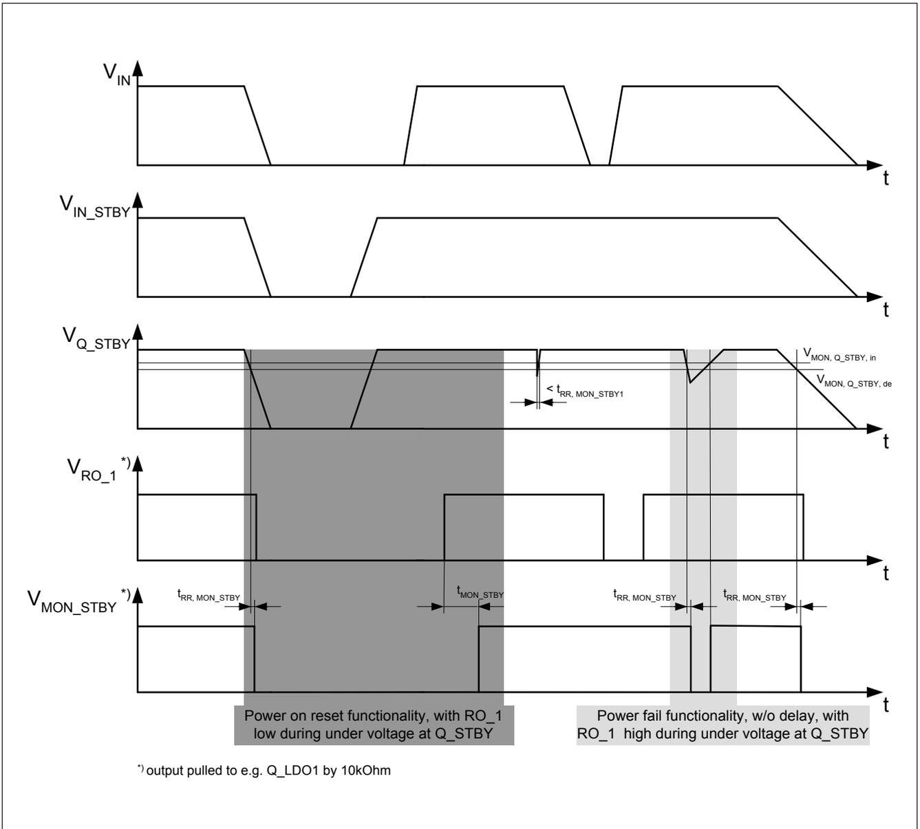
**Figure 7 Stand by Monitor Timing Diagram**
