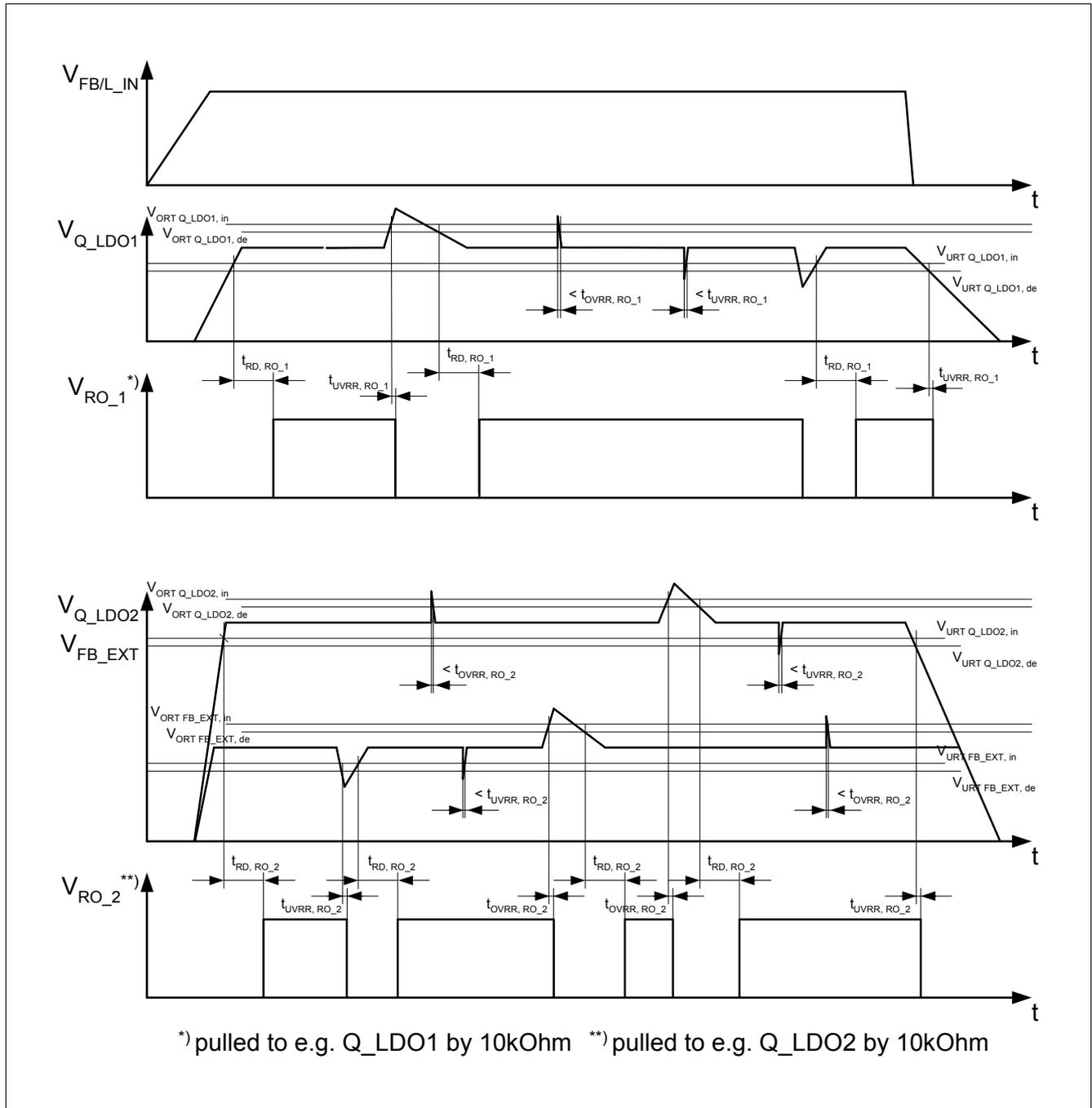
**Figure 5    Reset Timing TLE7368**
