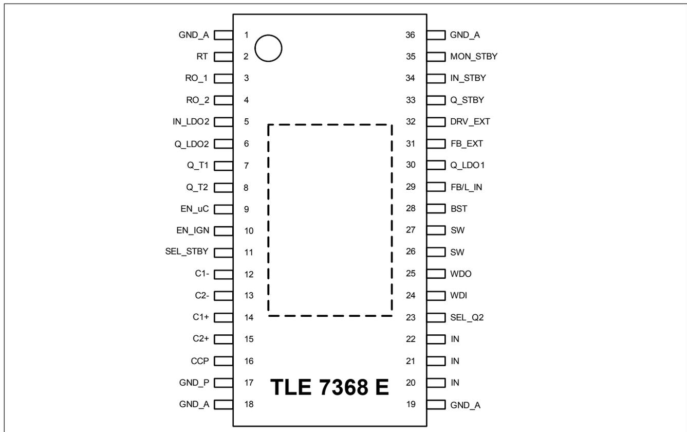
**Figure 2 Pin Configuration**
