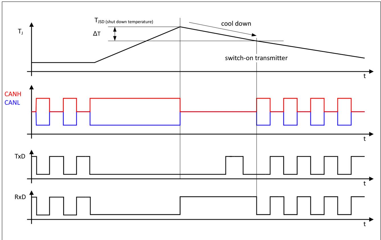
Figure 9 Overtemperature protection
