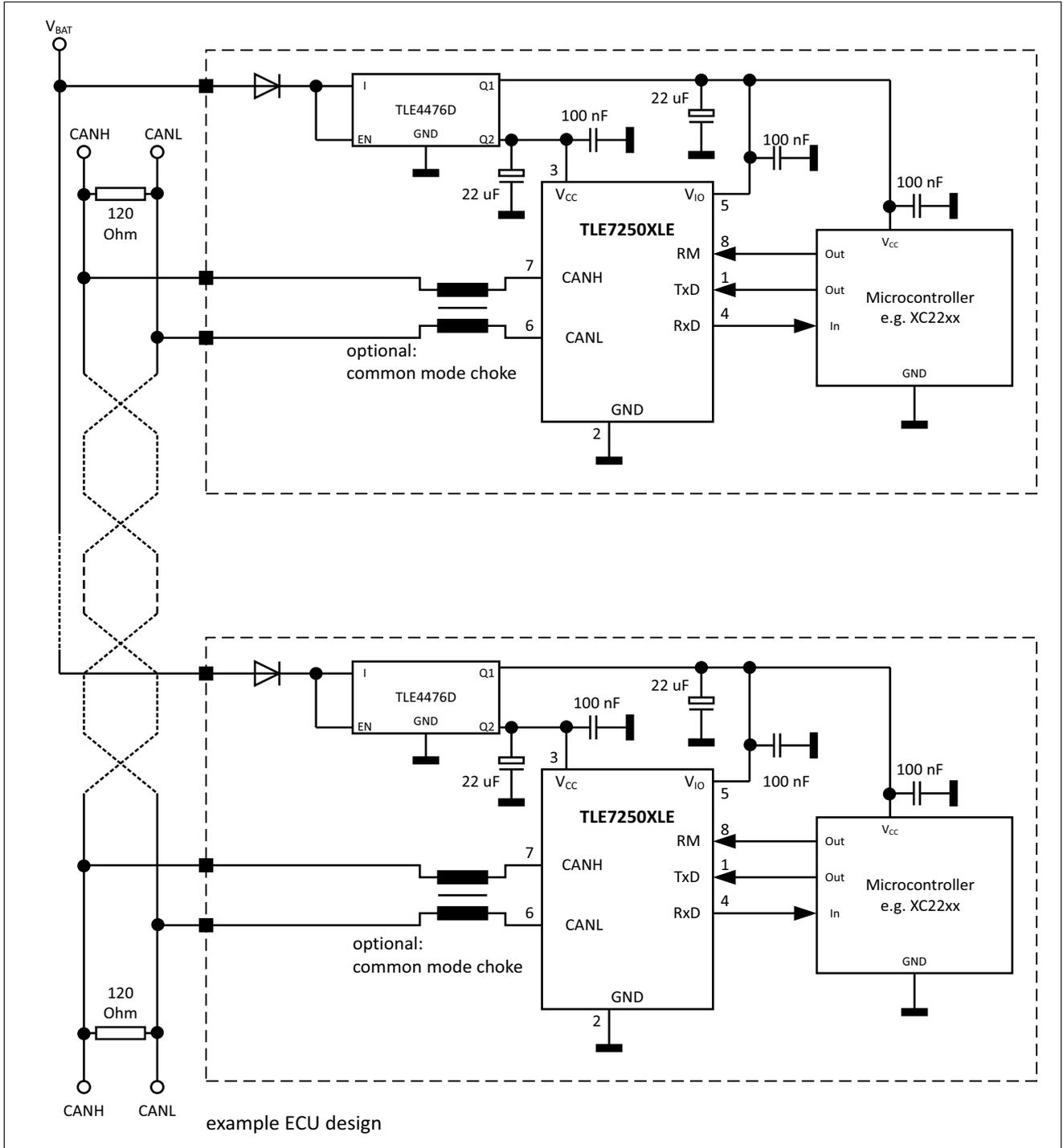
Figure 13 Application circuit
