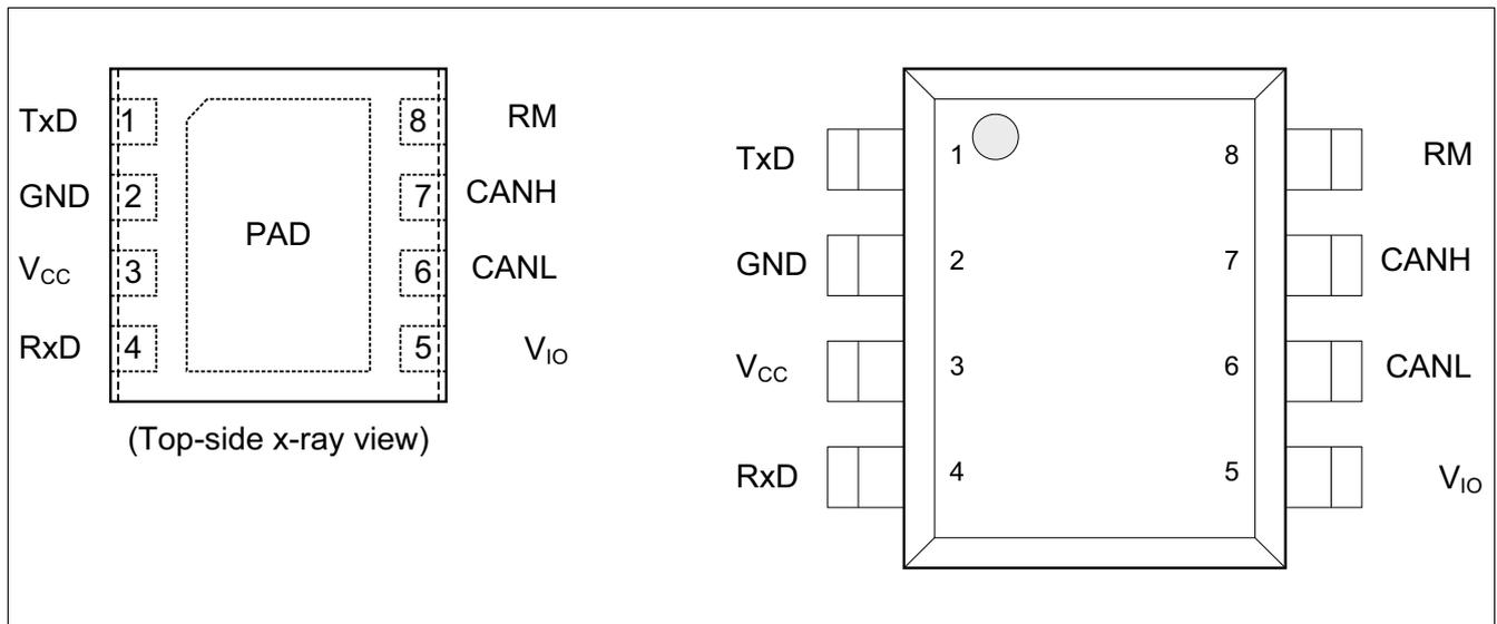
Figure 2 Pin configuration
