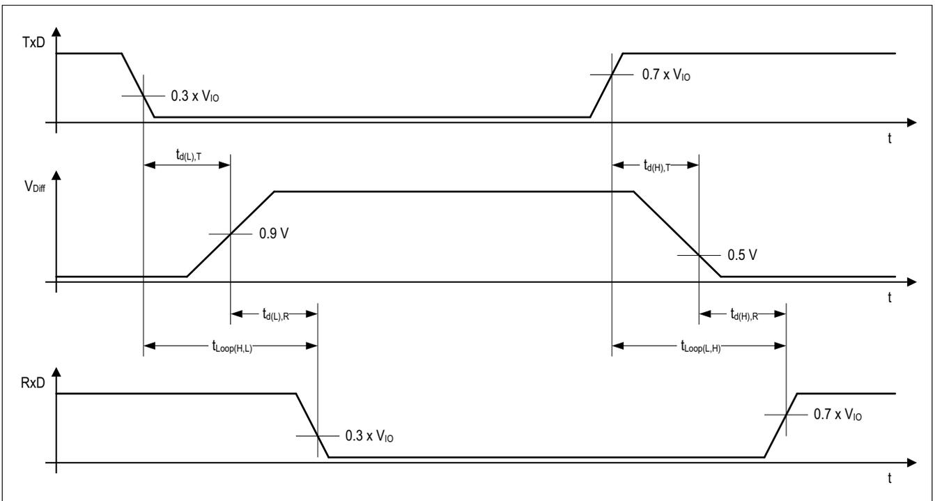
Figure 11 Timing diagrams for dynamic characteristics
