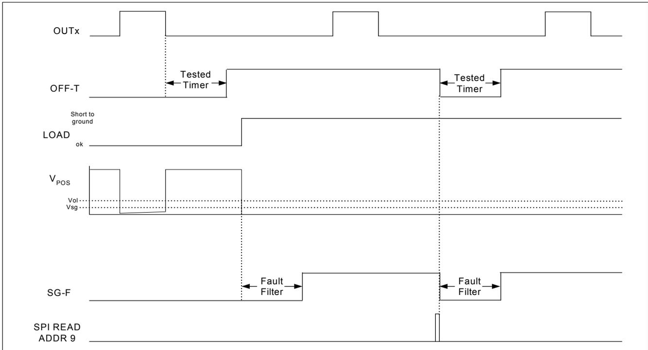
Figure 16 Off-State Diagnostics Timing Diagram - short to ground
