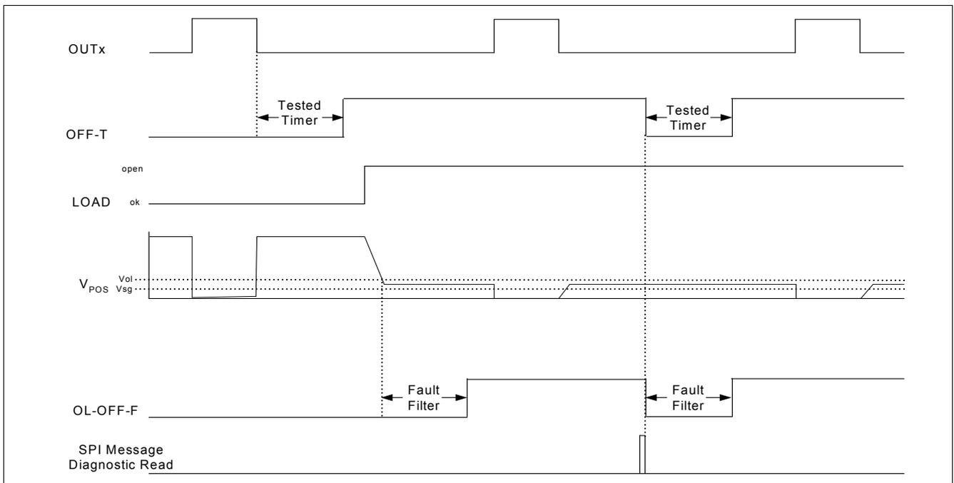
Figure 15 Off-State Diagnostics Timing Diagram - open
