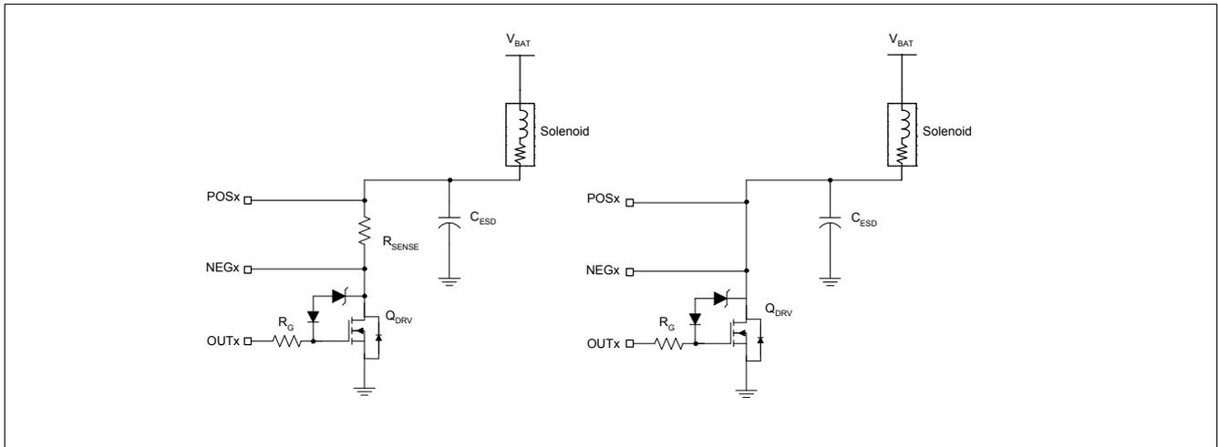
**Figure 1 External Circuit Diagram for On/Off Mode Operation**
