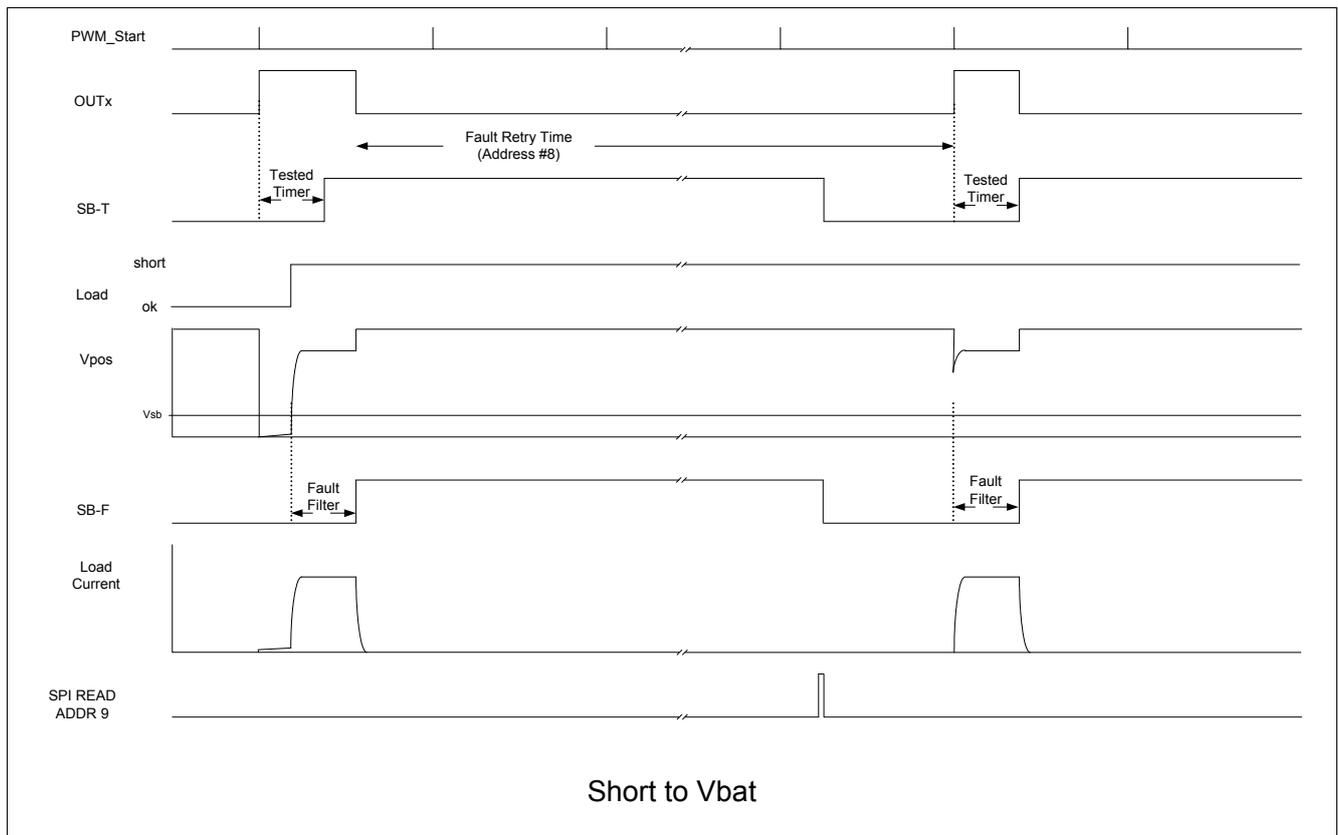
Figure 12 On-State Diagnostic Timing - Short to Vbat
