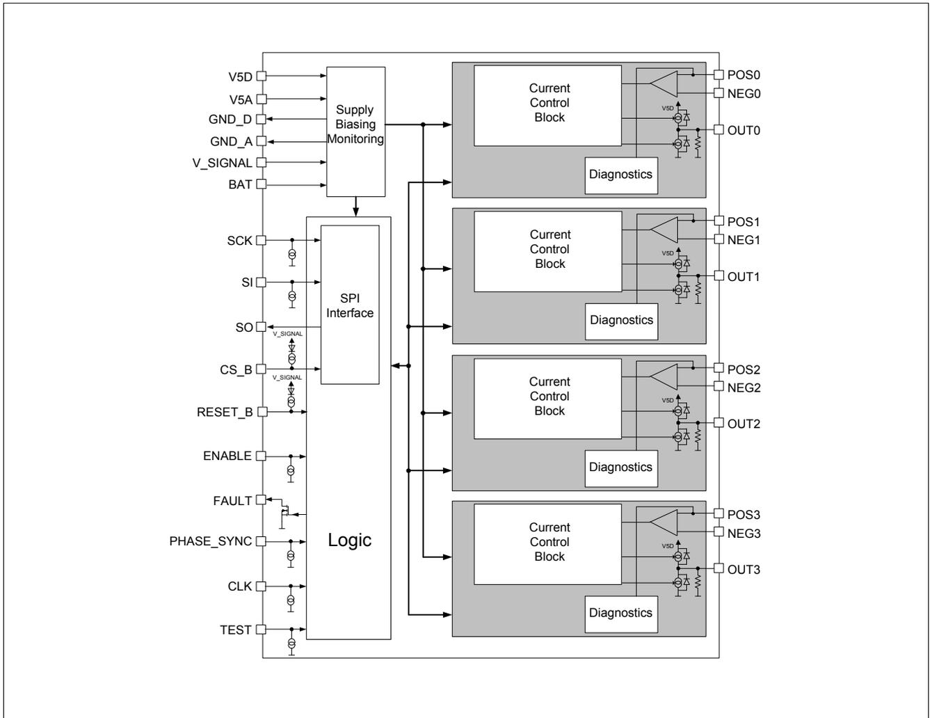
Figure 7 Block Diagram
