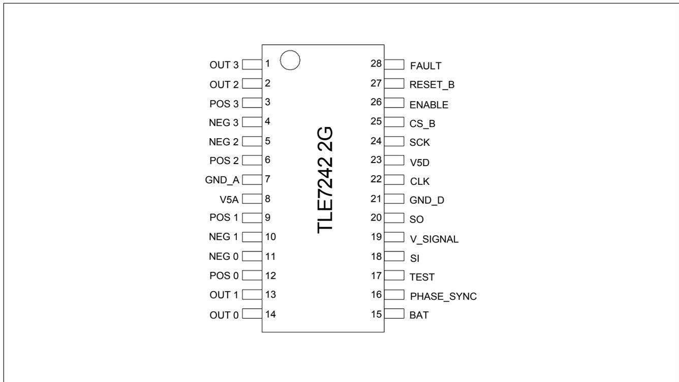
Figure 8 Pin Configuration
