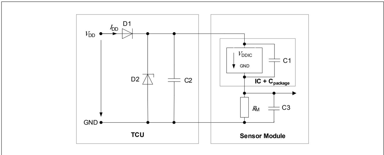
Figure 10 Application circuit
