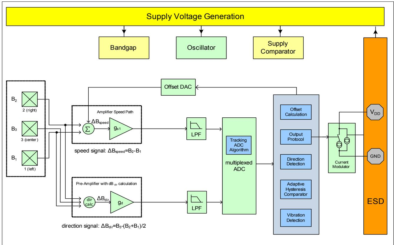
Figure 3 Block Diagram
