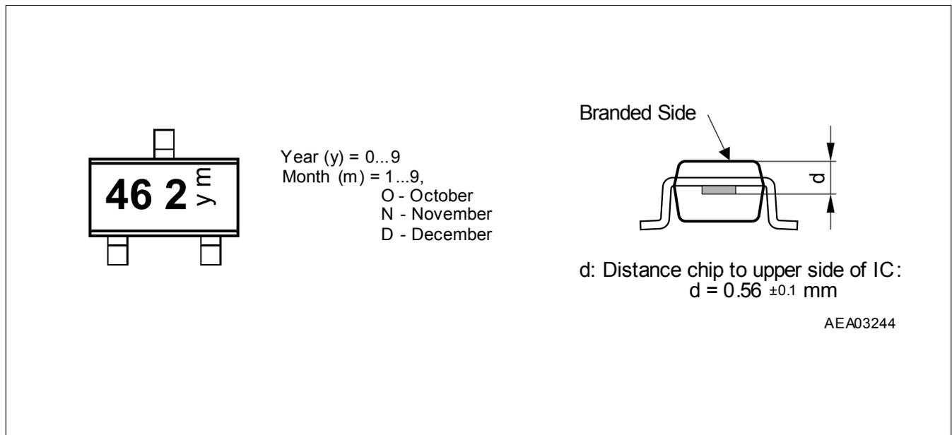
**Figure 5 Marking of TLE4946-2K and distance of chip to upper side of IC**
