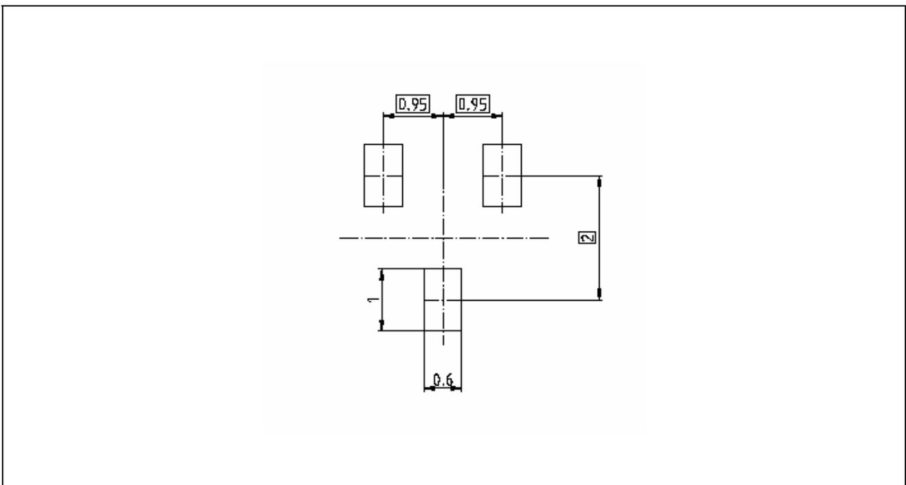
**Figure 6 Foot Print Reflow Soldering**
