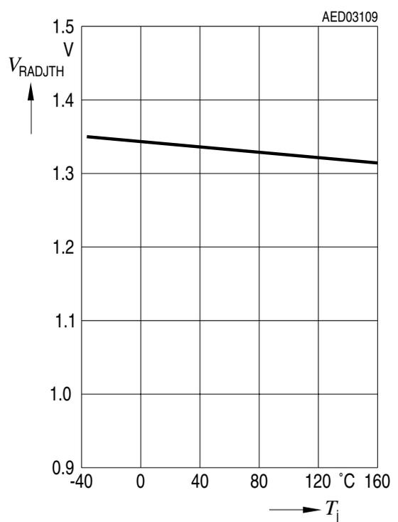
**Sense Threshold  $V_{Si}$  versus Temperature  $T_i$**
