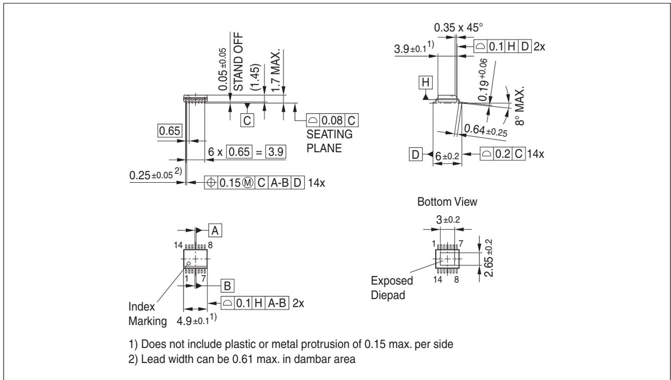
Figure 11 PG-SSOP-14 Exposed Pad<sup>1)</sup>
