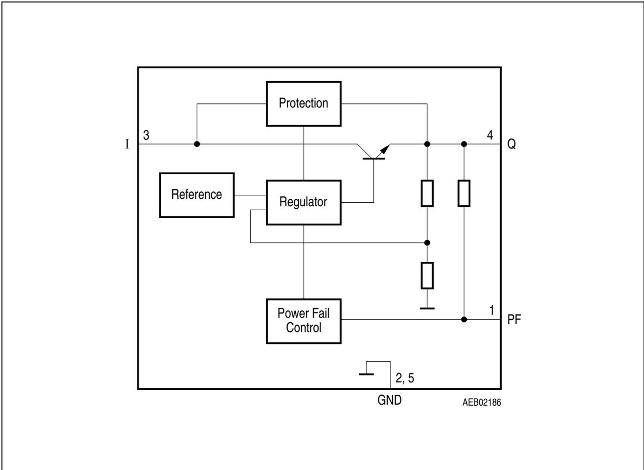
**Figure 2 Block Diagram**
