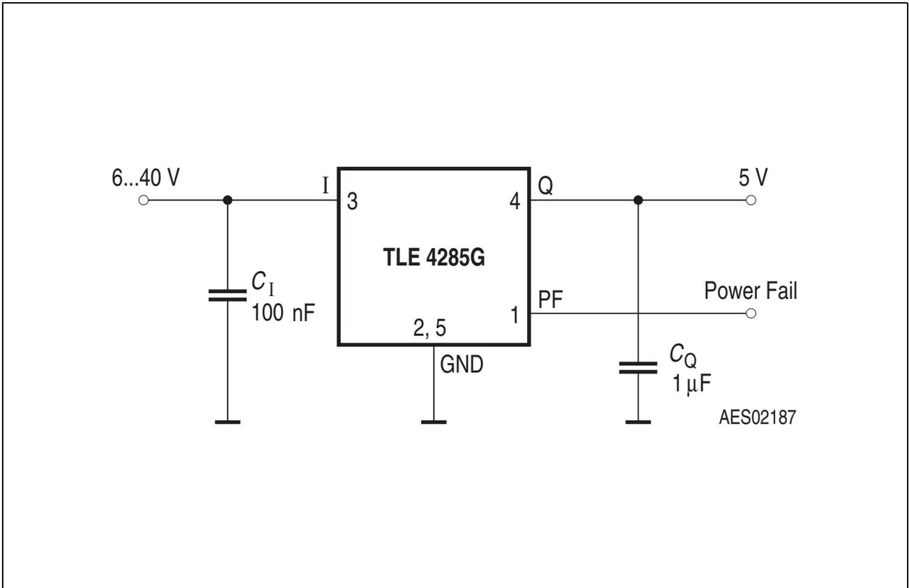
Figure 3 Application Circuit
