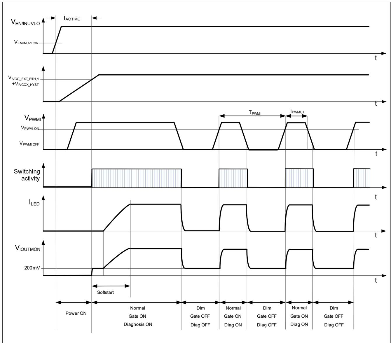
**Figure 13** Timing Diagram LED Dimming and Start up behavior example ( $V_{VDD}$  and  $V_{VIN}$  stable in the functional range and not during startup)
