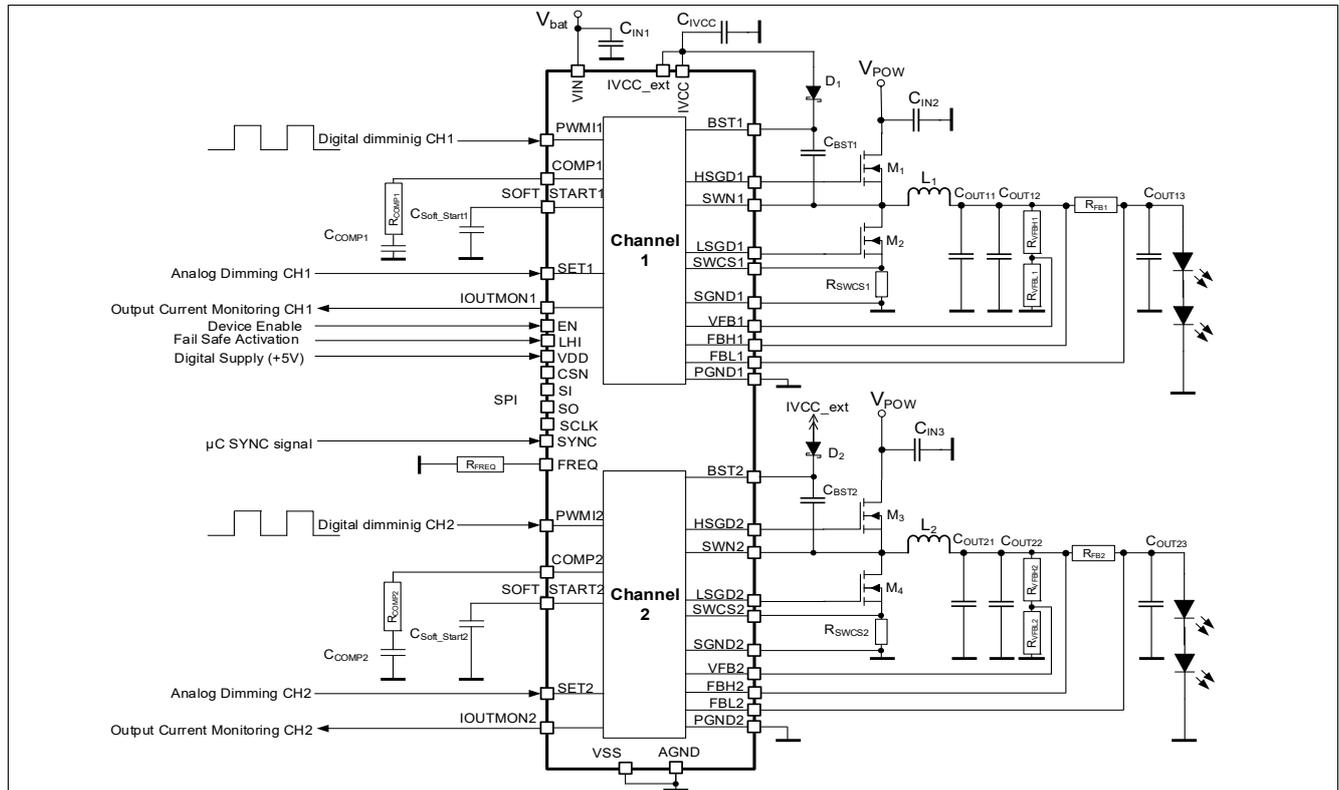
**Figure 37 Application Drawing - TLD5501-2QV as BUCK current Regulator, Separate Channels**
