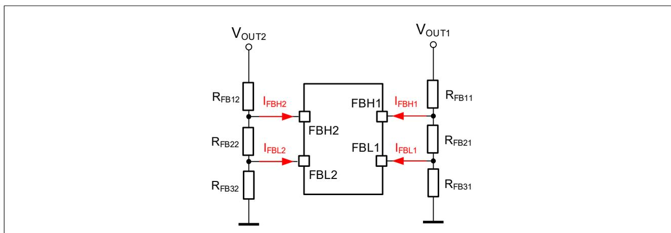
Figure 11 Programming Output Voltage (Constant Voltage Regulation)
