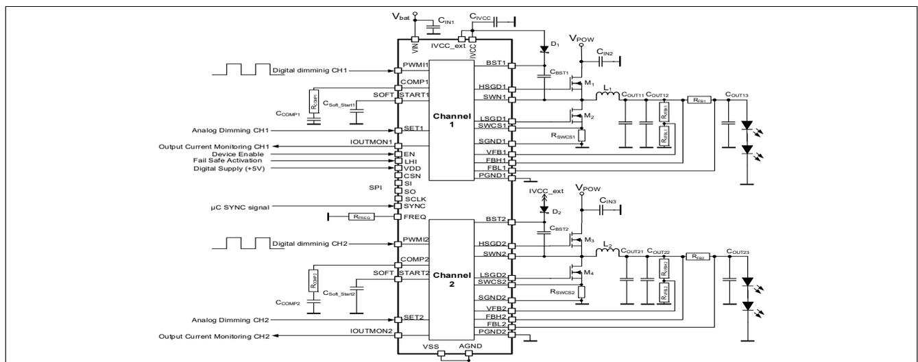
Figure 1 Application Drawing - TLD5501-2QV as current regulator
