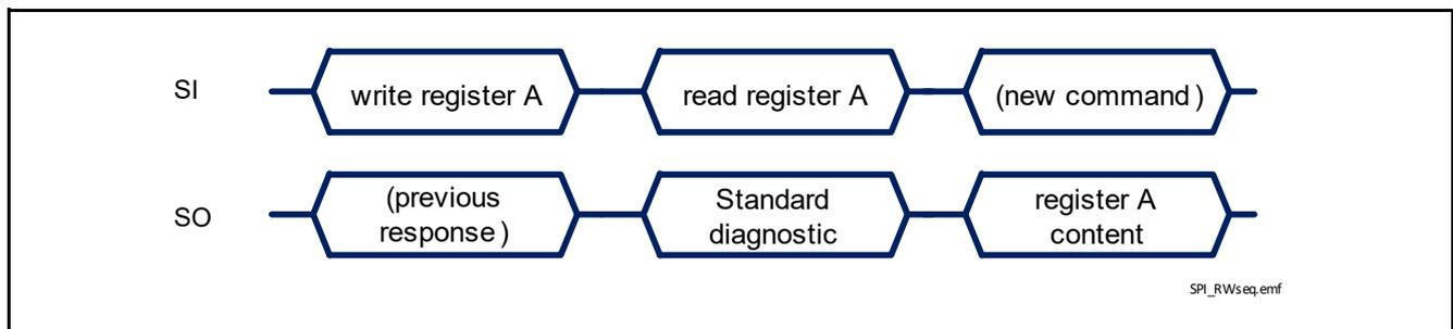
**Figure 34 Register content sent back to  $\mu\text{C}$**
