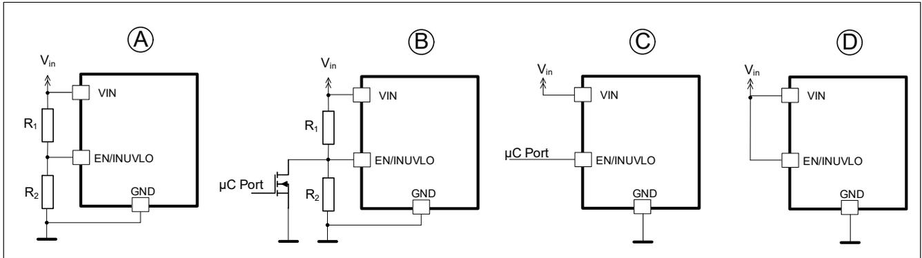
Figure 5 Usage of EN/INUVLO pin in different applications
