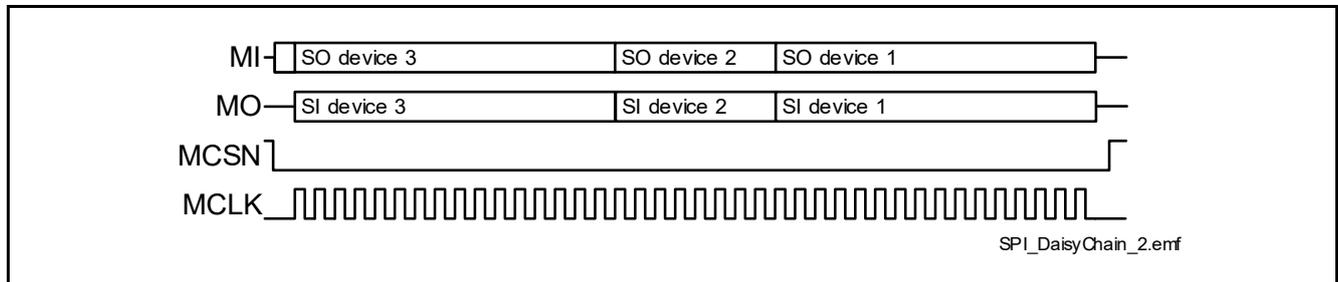
Figure 31 Data Transfer in Daisy Chain Configuration
