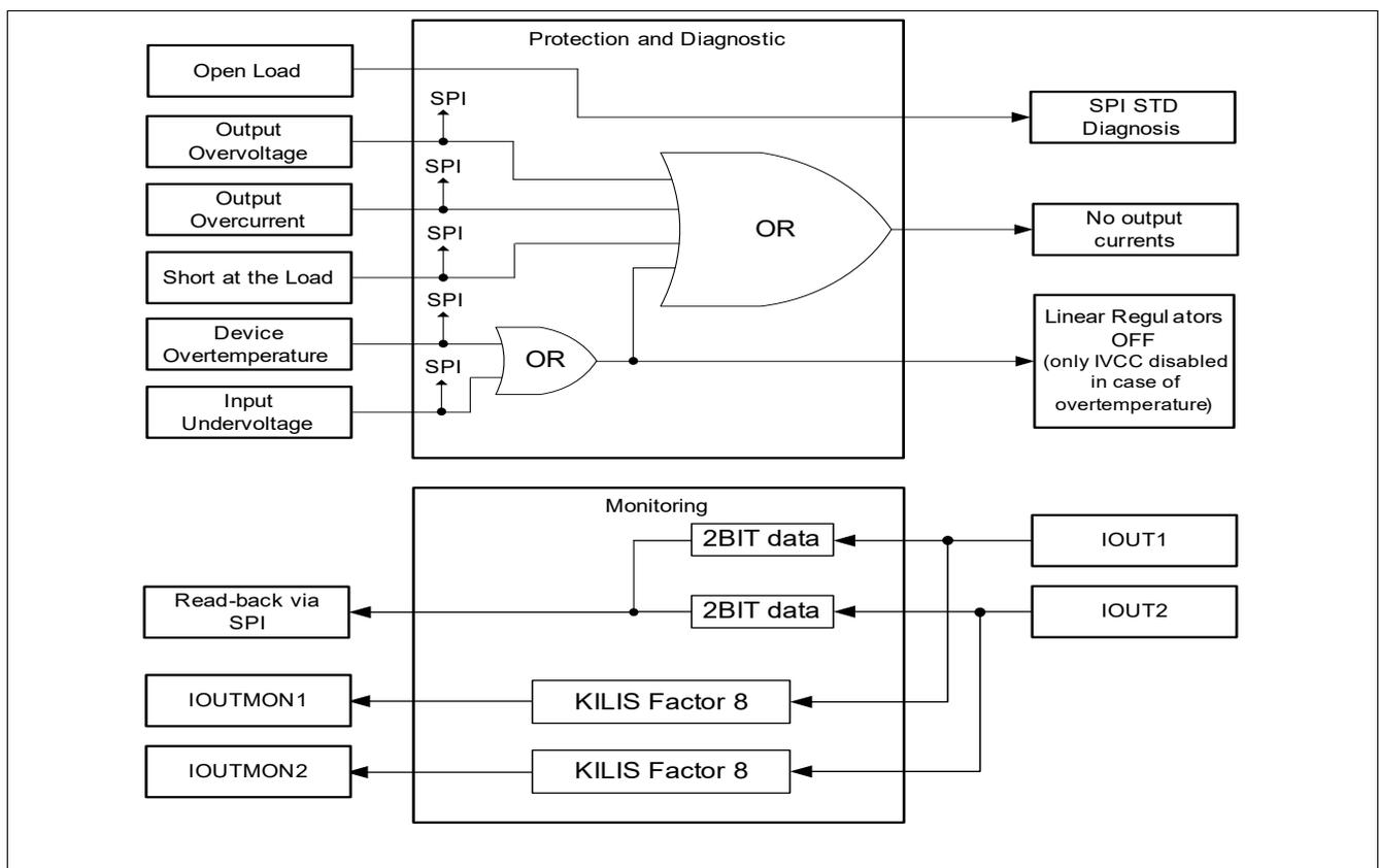
**Figure 20** Protection, Diagnostic and Monitoring Overview
