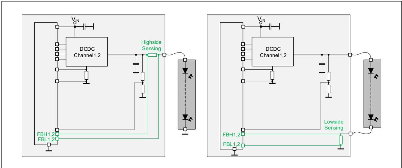
Figure 10 Highside and lowside current sensing - TLD5501-2QV
