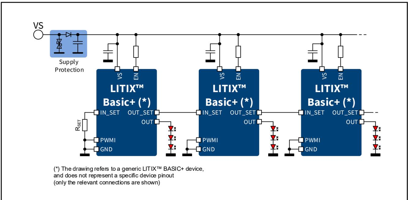
Figure 11 IN\_SET to OUT\_SET serial connection example
