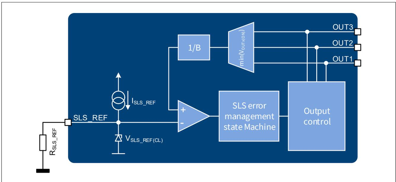
**Figure 22 SLS\_REF pin (block diagram) with resistor termination**
