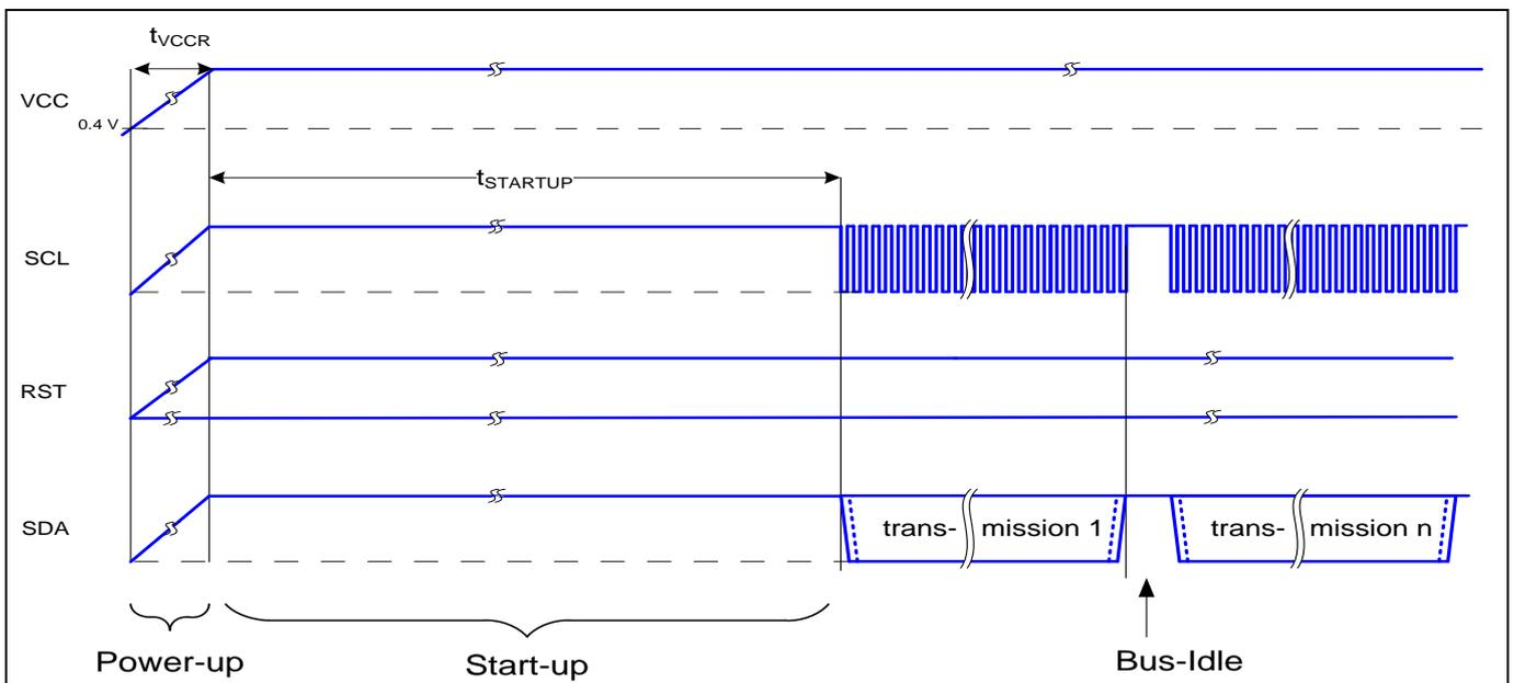
**Figure 8** **Startup of I2C Interface after Power-On**
