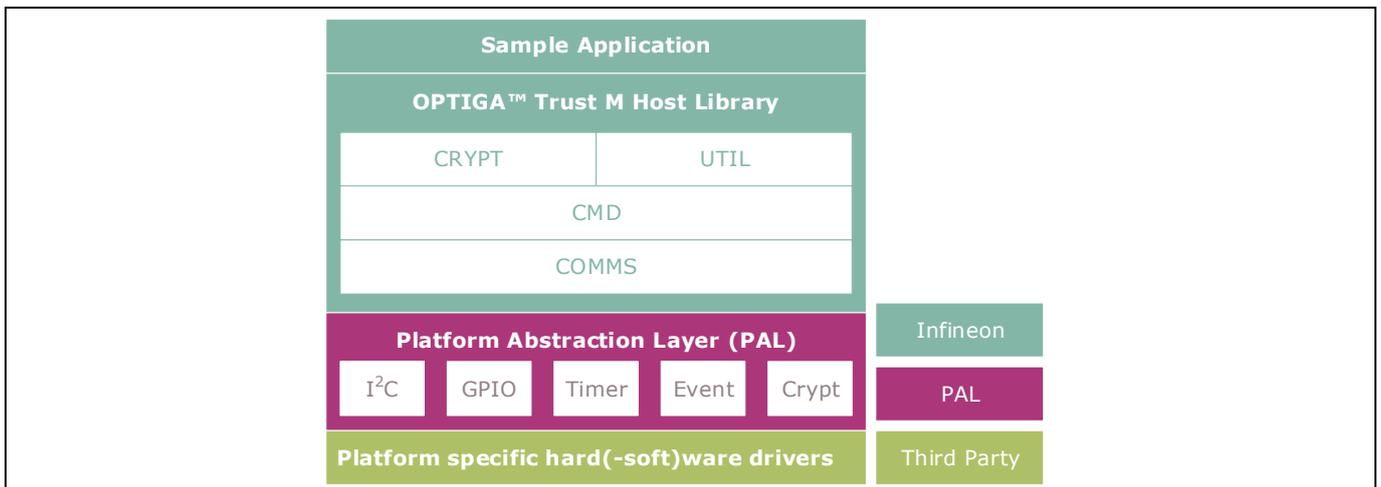
**Figure 10** OPTIGA™ Trust M Host Software Architecture
