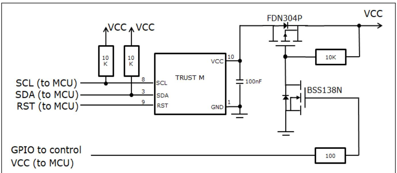
**Figure 3 System Integration Schematic Diagram with Hibernation**
