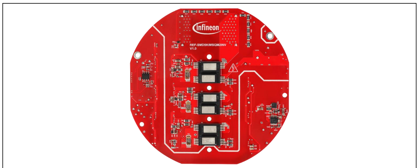
Figure 5 Power inverter board bottom
