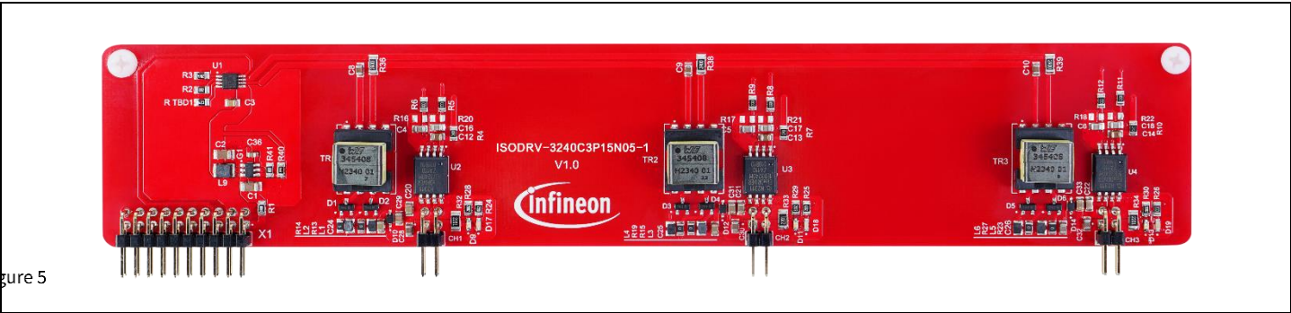
Gate driver board: ISODRV-3240C3P15N05-1
