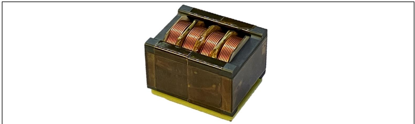
Figure 35 Finished common-mode choke prototype
