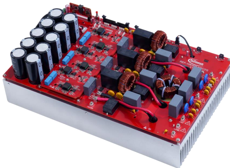
Figure 1 Power conversion board REF-10KW3LNPC2Q
