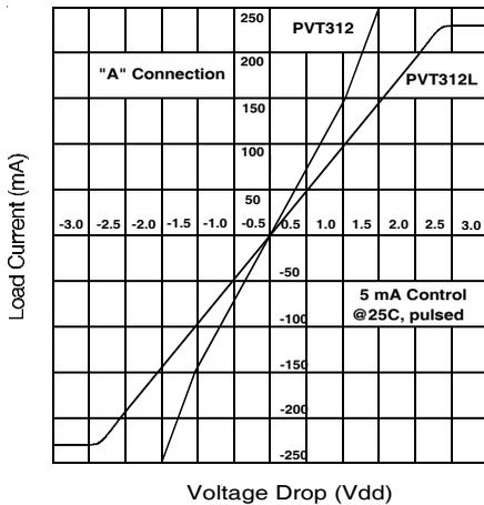
Figure 3. Linearity Characteristics
