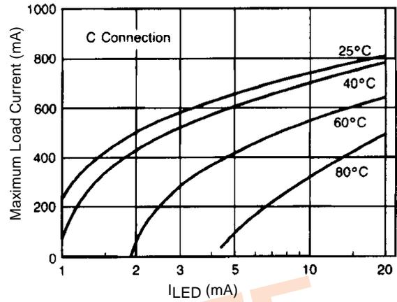
Figure 6. Typical Control Current Requirement (C Connection)
