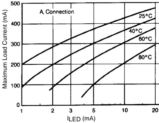
Figure 5. Typical Control Current Requirement (A Connection)
