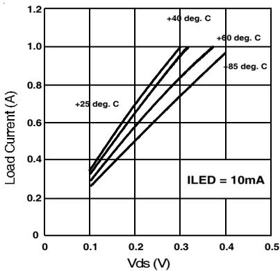
**Figure 3. Typical On-Characteristics**
