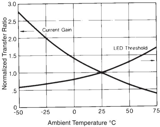
Figure 9. Typical Control Threshold and Transfer Ratio
