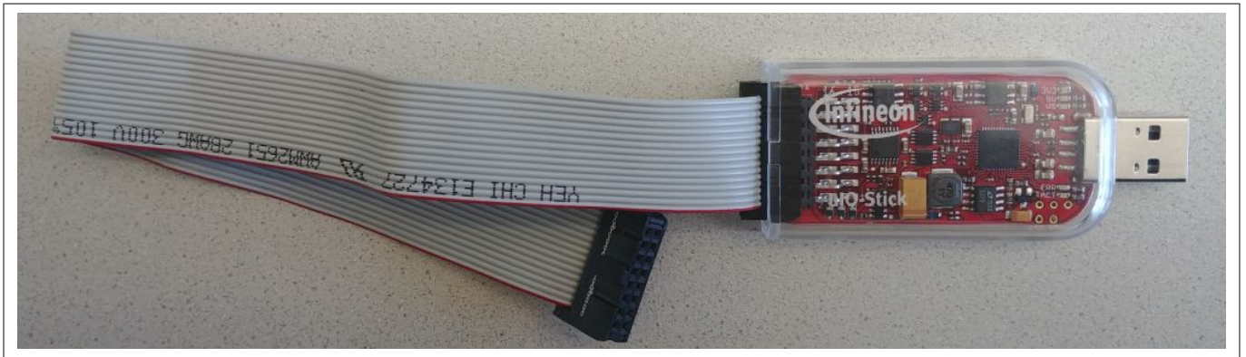
Figure 31 Infineon \mu IO-Stick with ribbon cable
