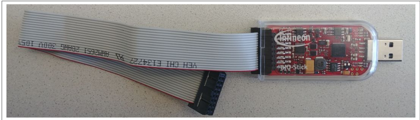
Figure 37 Infineon µIO-Stick with ribbon cable
