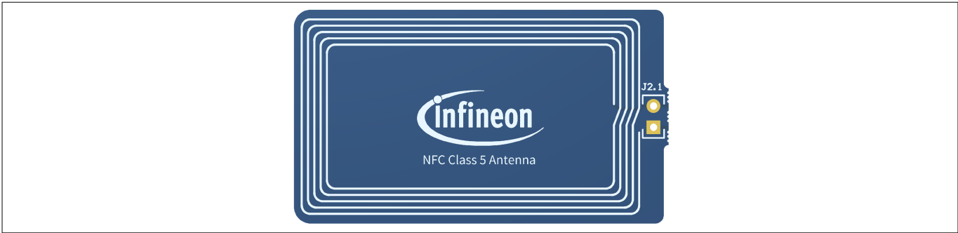
Figure 5 Board details of the Class 5 shield antenna
