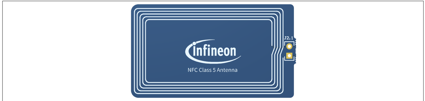
Figure 5 Board details of the Class 5 shield antenna
