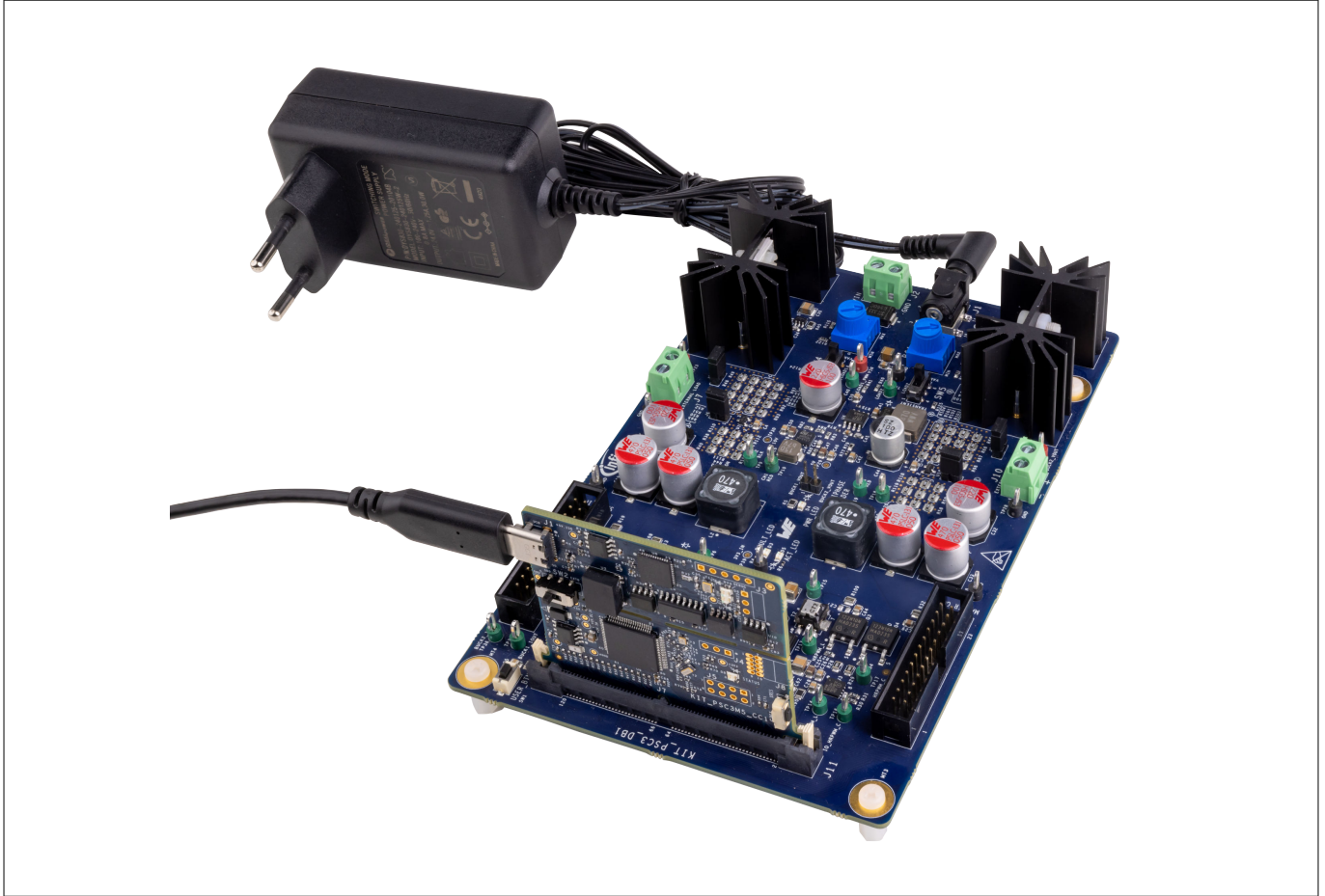
Figure 3 Complete setup with Control Card and Dual Buck Evaluation Board
