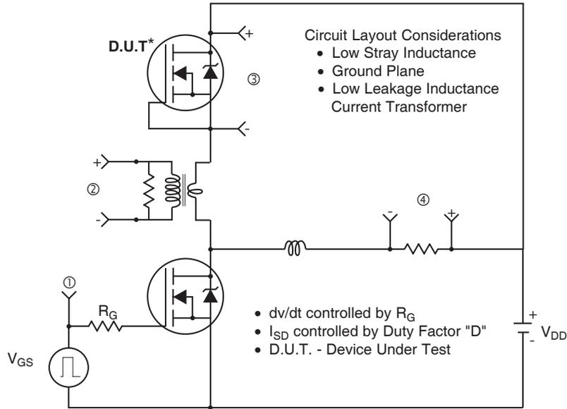
\* Reverse Polarity of D.U.T for P-Channel
