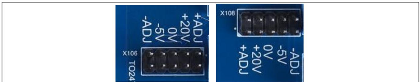
Figure 6 Drive voltage jumpers
