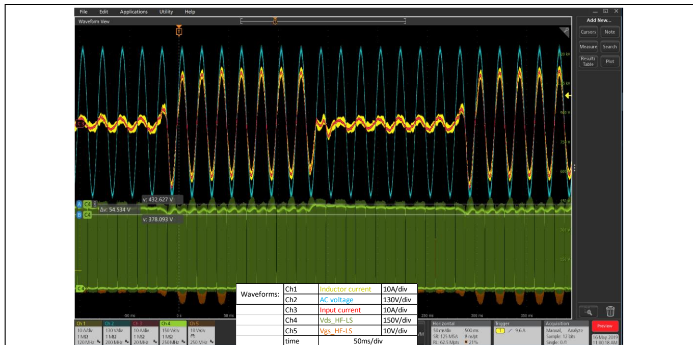
Figure 19 3.3 kW SiC totem-pole CCM PFC response for 10 percent to 90 percent load steps every 150 ms with 0.2 A/μs current slope
