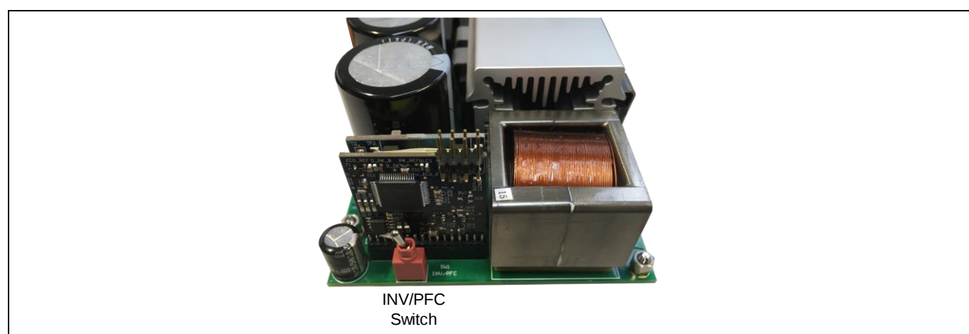
Figure 26 Switch to select the operation mode (PFC or inverter) in EVAL_3K3W_TP_PFC_SIC2
