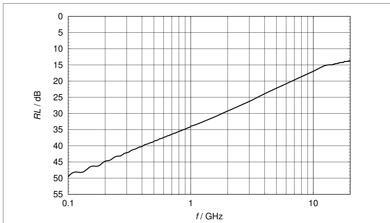
Figure 10 Return loss R_L = f(f) , measured in a 50 \Omega system
