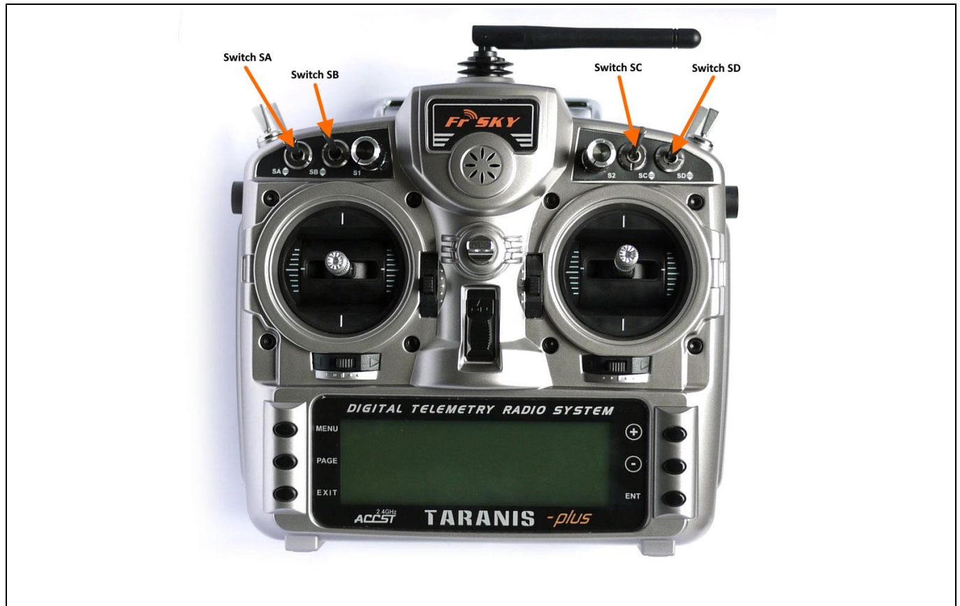
Figure 27 Taranis X9D+ digital telemetry radio system – remote control
