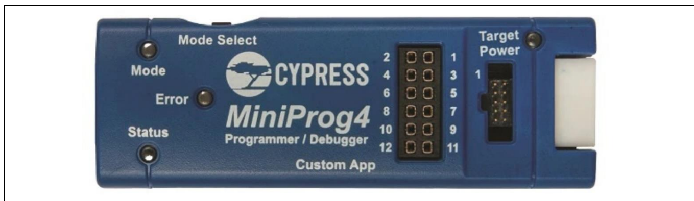
Figure 12 MiniProg4 Program and Debug Kit (CY8CKIT-005)
