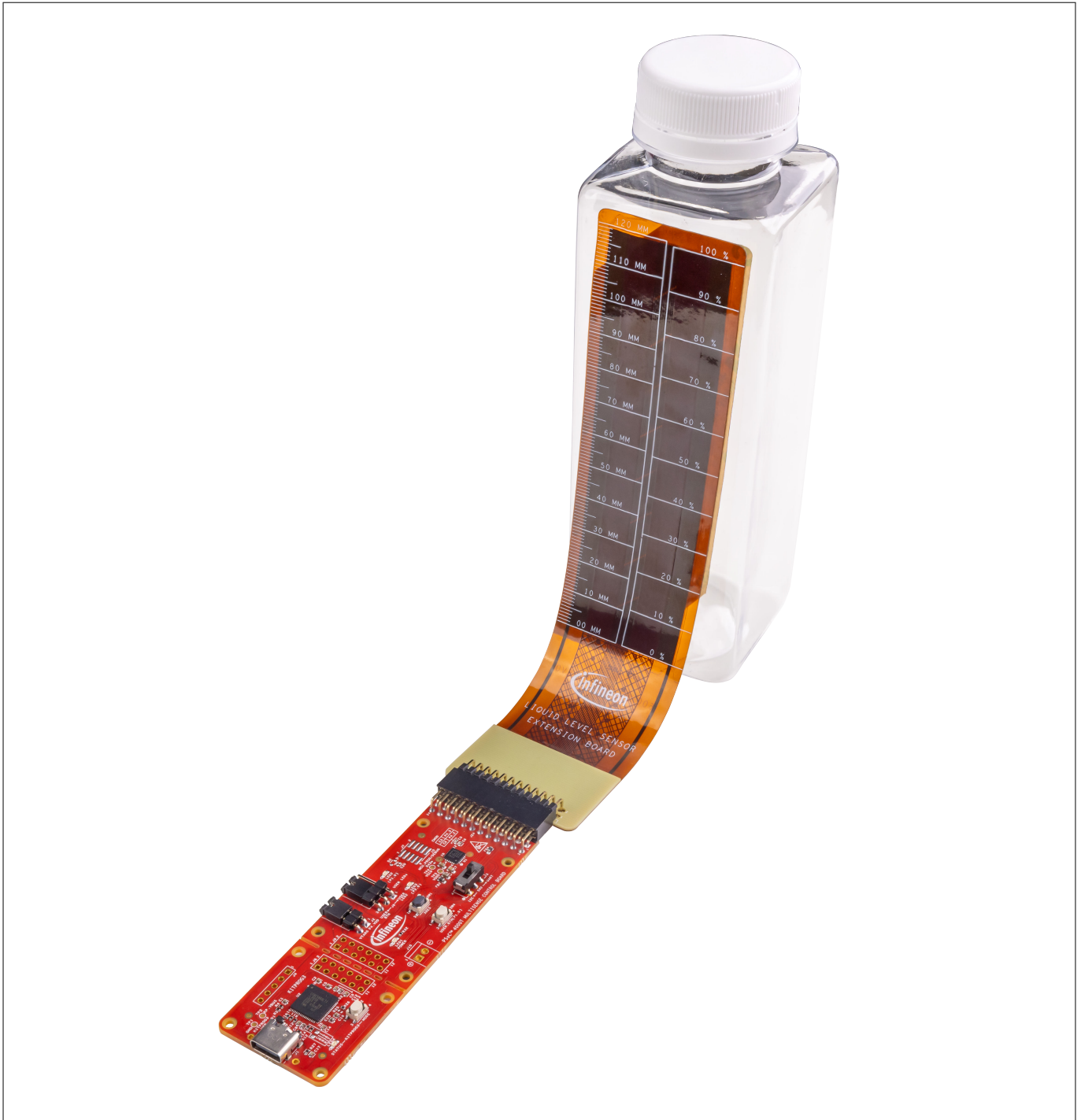
Figure 54 Liquid level sensing setup with container
