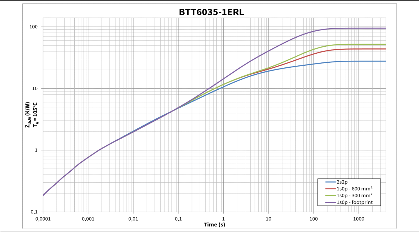
Figure 7 Typical Thermal Impedance. 2s2p set-up according Figure 5
