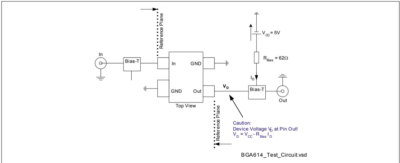
Figure 2 Test Circuit for Electrical Characteristics and S-Parameter
