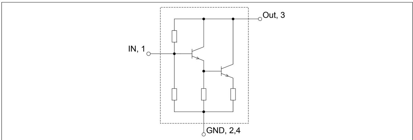
Figure 1 Pin connection
