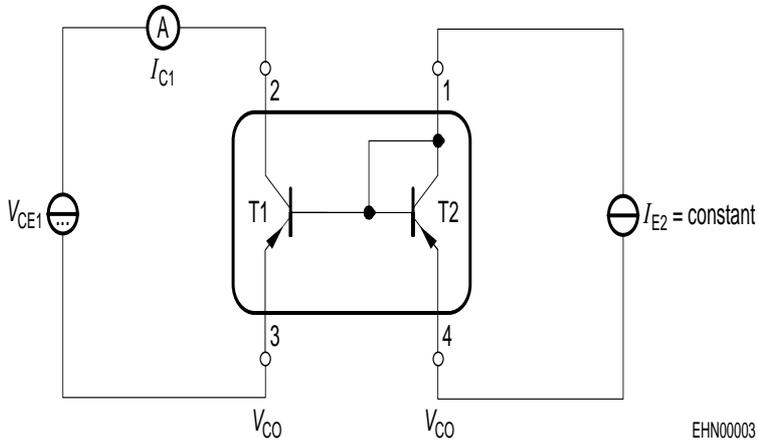
Note: Voltage drop at contacts:  $V_{CO} < 2/3 V_T = 16\text{mV}$
