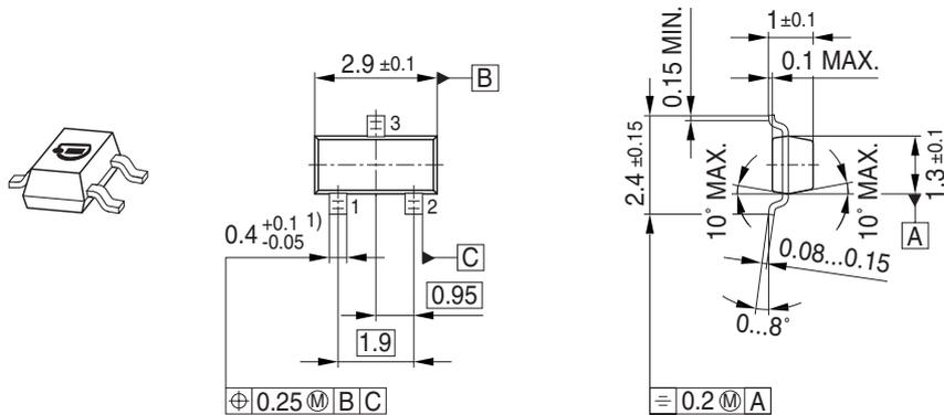
1) Lead width can be 0.6 max. in dambar area
