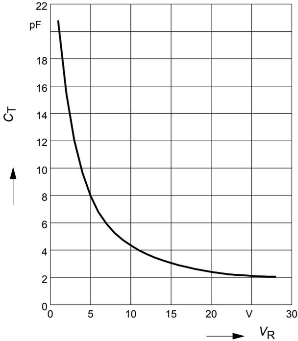
**Normalized diode capacitance**
