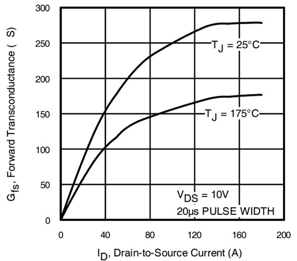
Fig. 4 Typical Forward Transconductance vs. Drain Current
