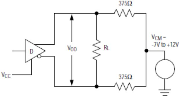
Figure 2. Driver  $V_{OD}$  with Varying Common-Mode Voltage
